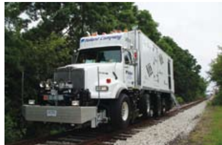
Figure 4B: TrackStar Hi-Rail Inspection Vehicle 3
