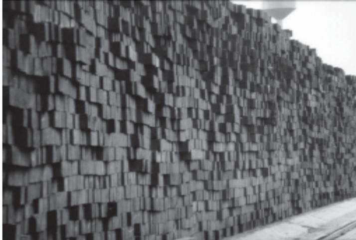
been treated with a creosote solution meeting the requirements of AWPAs Standard P2. There are also occasions when ties and other timber products such as bridge materials will be treated using the AWPAs Standard P1/P13 .
