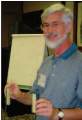
Basically, you add the preservative (or in this case water colored with green food coloring—er, uhh—pickle juice), apply pressure and voila—treated wood! Note how in this five-minute experimental classroom approach to wood treating how easily the sapwood section of the sample block treated.
