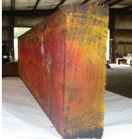
Fig. 7 White Oak Cross Section Boron Rod Diffusion
