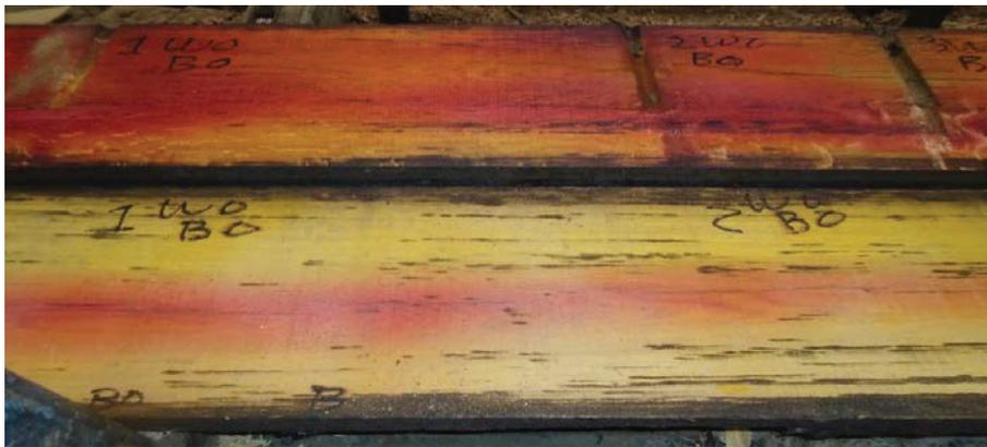
Fig.8 White Oak Boron Rod Diffusion Top Board(C)
