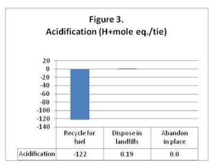
methane combustion and abandoning ties has no impact to acidification.
