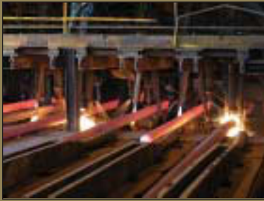
As the steel runs out onto a table for more cooling, it is cut by a torch into "blooms."
