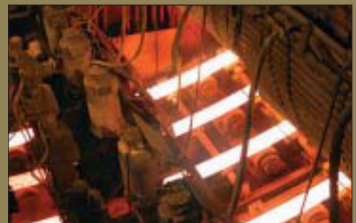
Saying that the steel has already cooled is relative. Here, as it traverses a vertical drop, it is still red hot. The push rollers on the left push against the enormous weight to control the descent.
