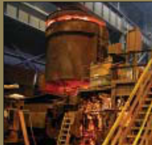
This is followed by the ladle being received at the tundish...
