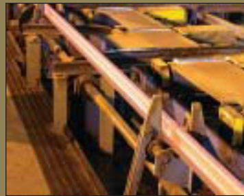
Rocky Mountain Steel is one of the few—if not the only rail maker—that has instituted quality control procedures while the rail is still hot. On this bed, several measurements are made intermittently as rail is formed from blooms.
