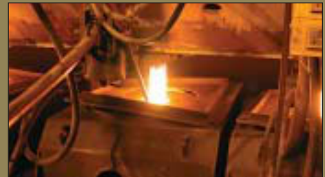
...where the molten steel is measured carefully through a ceramic tube into a water-cooled jacket where it undergoes the first step in cooling as the strands of steel are created.
