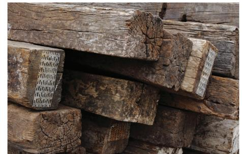
Storing used rail ties in the manner pictured above is not allowed in California. Hazardous waste should be stored, handled and transported under California regulations that prevent water runoff from the wood into the environment.
