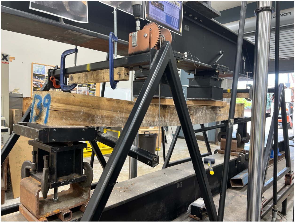
Figure 2. Demonstration of static bending test in Instron 600 kN capacity universal testing machine.
