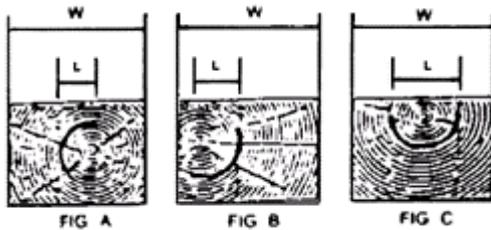
The procedure illustrated in the above diagrams shall be used in determining the length of a shake. One which is not more than 1/3 the width of the tie will be allowed, provided it does not extend nearer than 1" to any surface.
