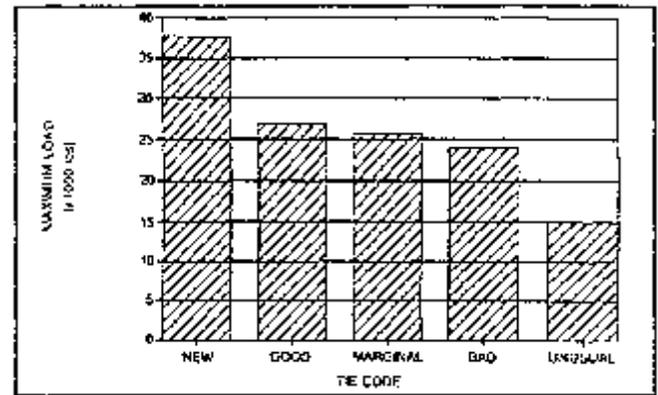
Figure 1 - Maximum static bending load for 20-year-old ties (1).
