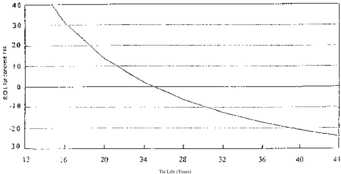
Figure 3 - Economic benefit analysis. wood vs. concrete ties (based on assumptions indicated).
