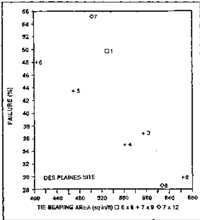
Figure 1 - Failure rate vs. tie bearing area
