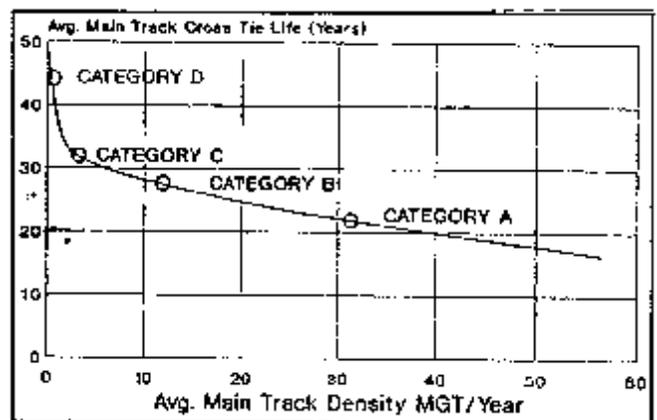
Figure 2 - Tie life versus tonnage, from 1978 industry statistics<sup>2</sup>
