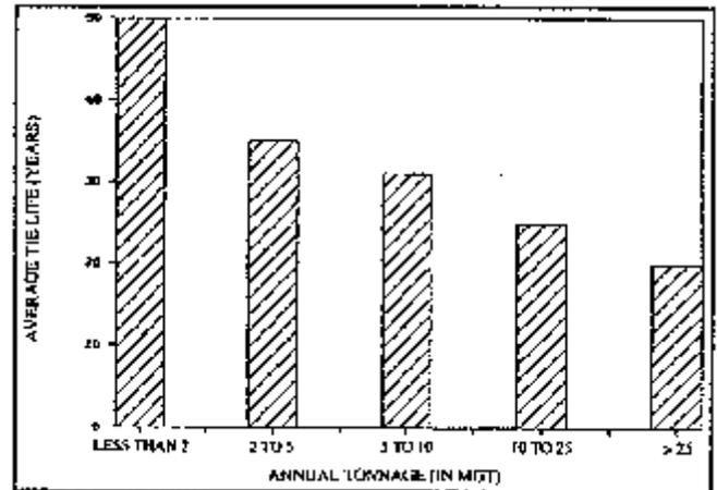
Figure 1 - Average tie life (data from 1934 to 1957)<sup>1</sup>
