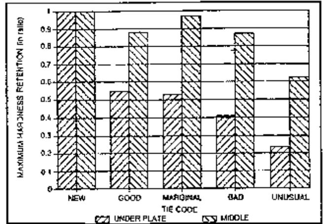
Figure 4 - Maximum hardness retention for 20-year-old ties (1).
