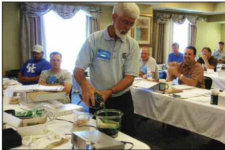
Conners, using his "magic pickling juice" (water with green food coloring) and a vacuum pump, illustrates how sapwood of many species is very easily treated while the heartwood of those same species is harder to penetrate with wood preservatives.
