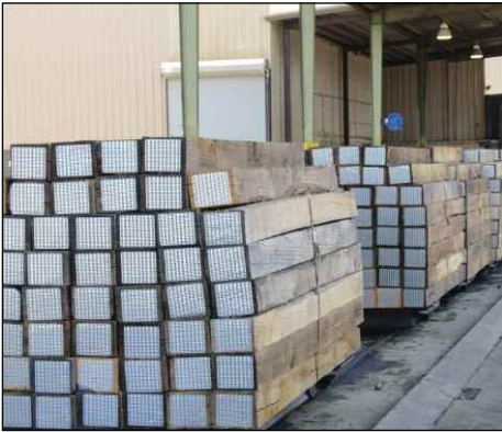
After conditioning, the ties are loaded onto trams for creosote treatment in one of two pressure vessels.
