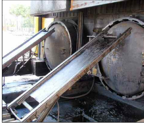
After conditioning, the ties are loaded onto trams for creosote treatment in one of two pressure vessels.
