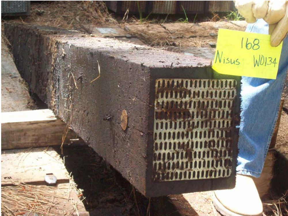
Figure 21- Tie #168 (Nisus/white oak/borate/oil A).
