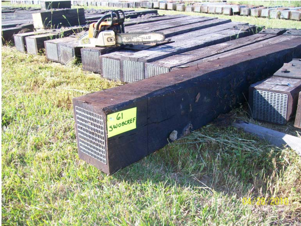
Figure 13 - Tie #61 (Boatright/white oak/borate/creosote to refusal).
