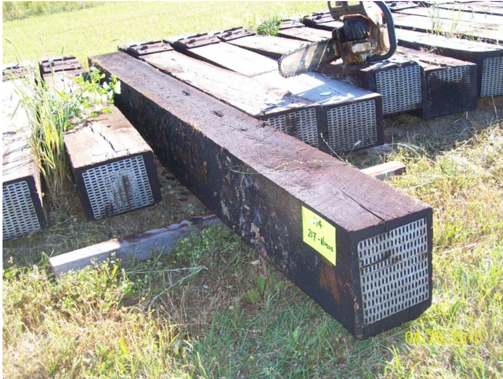
Figure 26 - Tie #114 (Nisus/white oak/borate/oil B).
