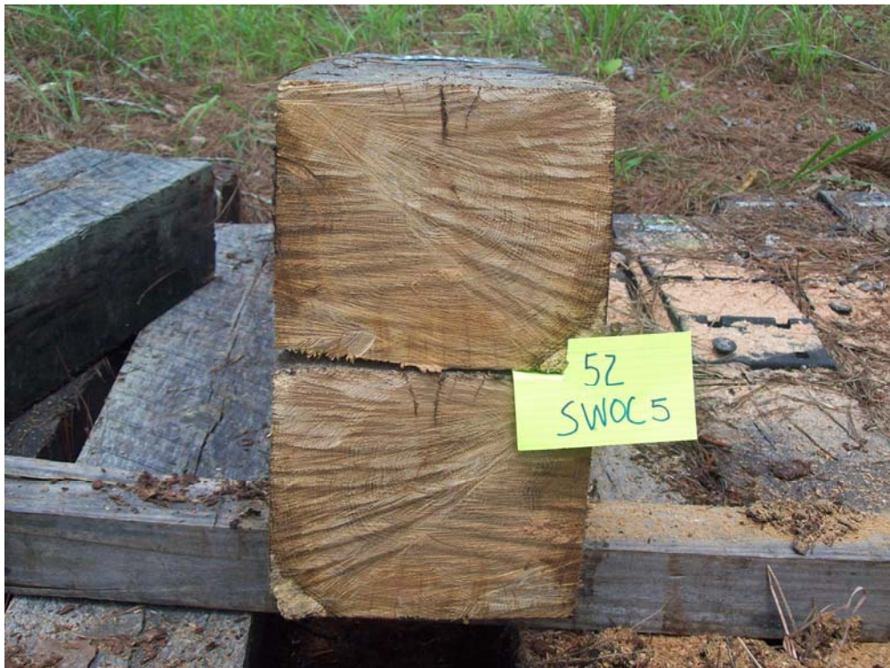
Figure 52 - Tie #52 (Boatright/white oak/untreated control).
