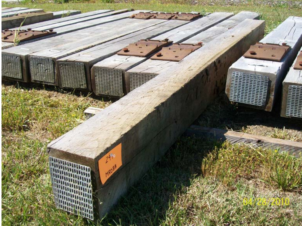
Figure 48 - Tie #241 (Merichem/red oak/borate/CuNap).
