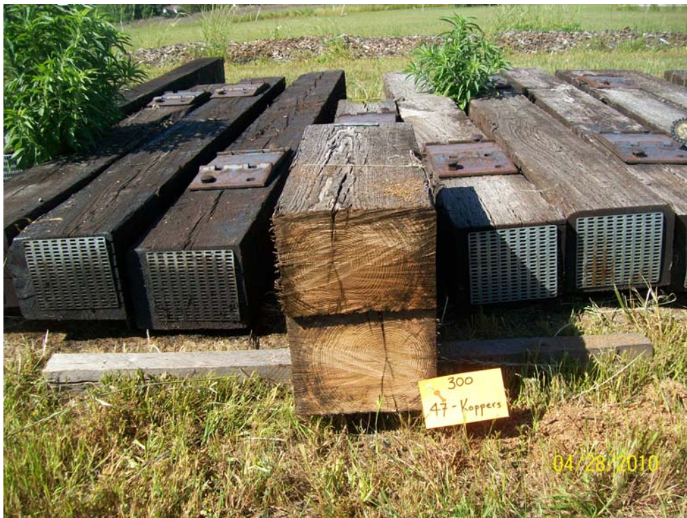
Figure 41 - Tie #300 (Koppers/red oak/creosote petroleum solution).
