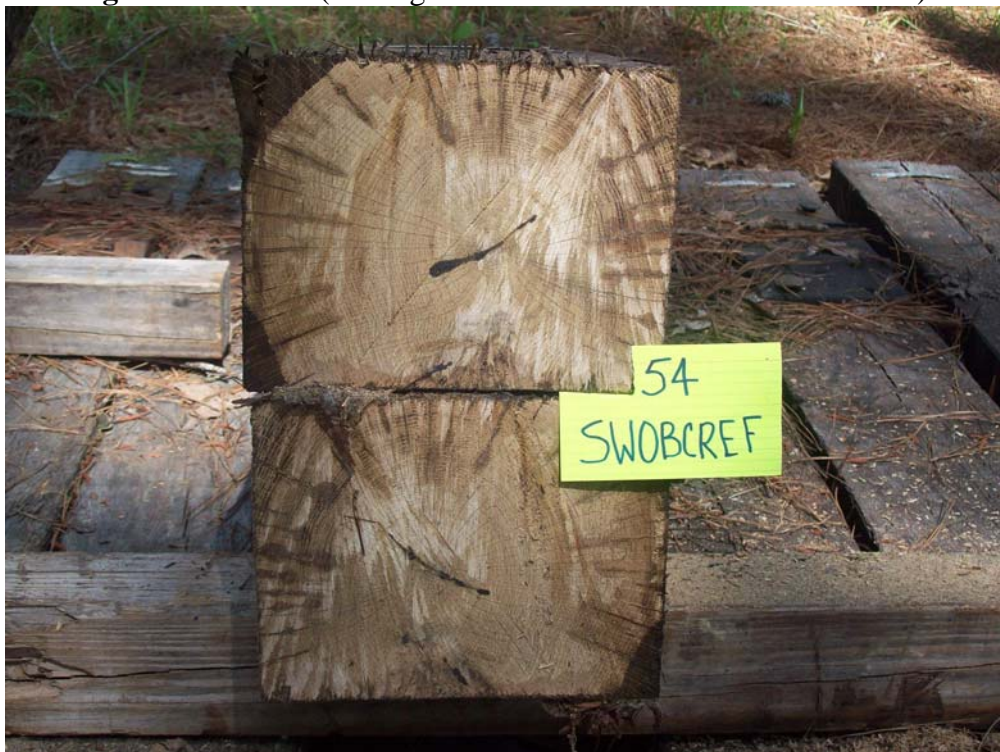
Figure 48 - Tie #54 (Boatright/white oak/borate/creosote to refusal).
