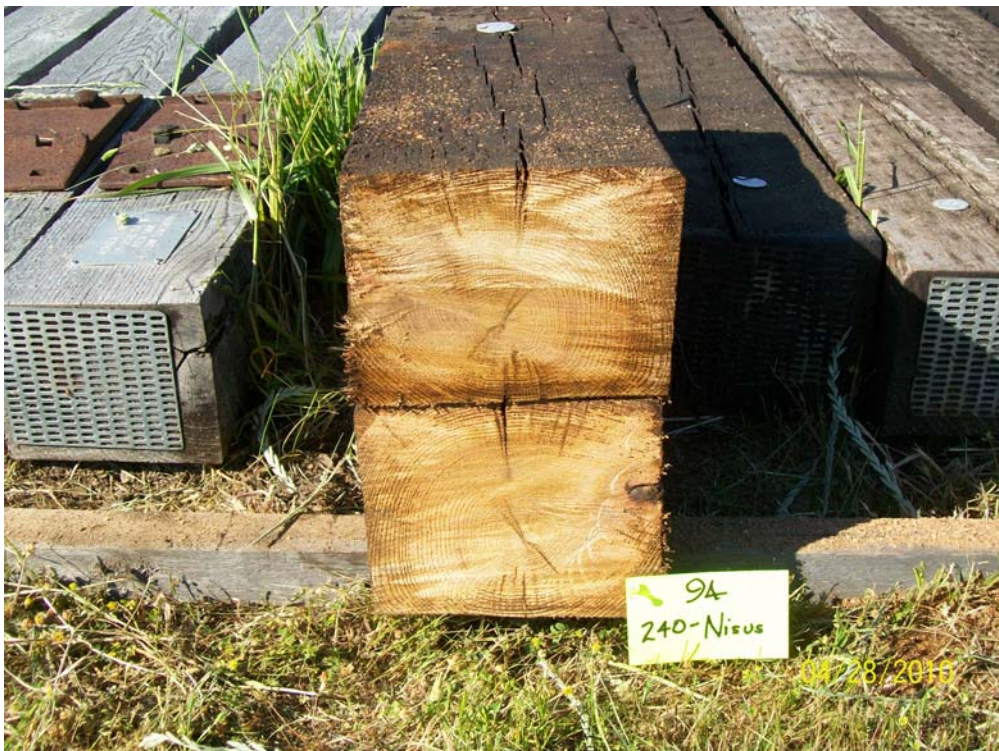
Figure 23 - Tie #94 (Nisus/red oak/borate/oil A).
