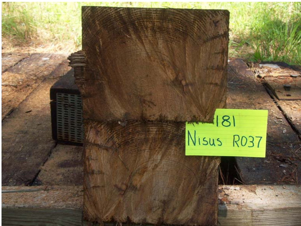
Figure 28 - Tie #181 (Nisus/red oak/borate/oil A).
