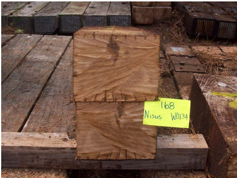
Figure 22 - Tie #168 (Nisus/white oak/borate/oil A).
