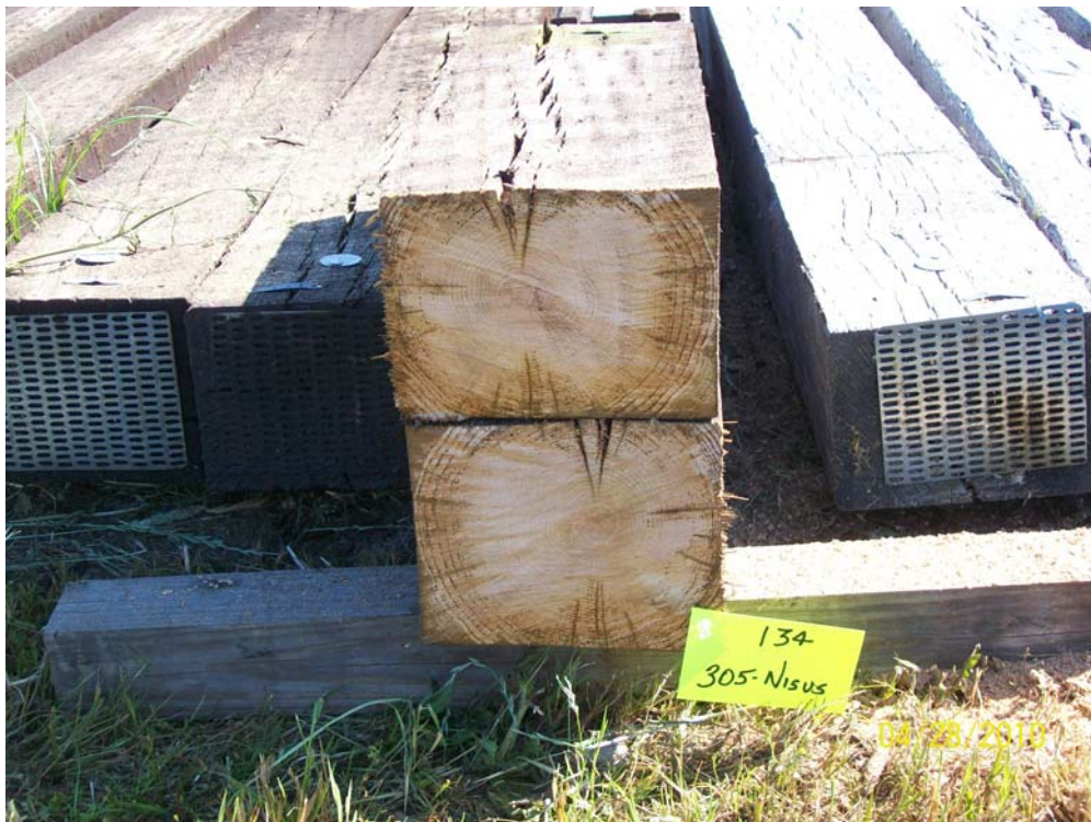
Figure 31 - Tie #134 (Nisus/white oak/borate/oil A).
