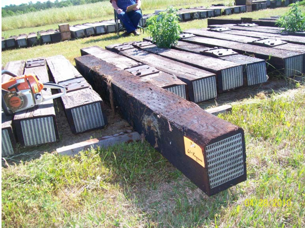
Figure 38 - Tie #310 (Koppers/white oak/creosote petroleum solution).
