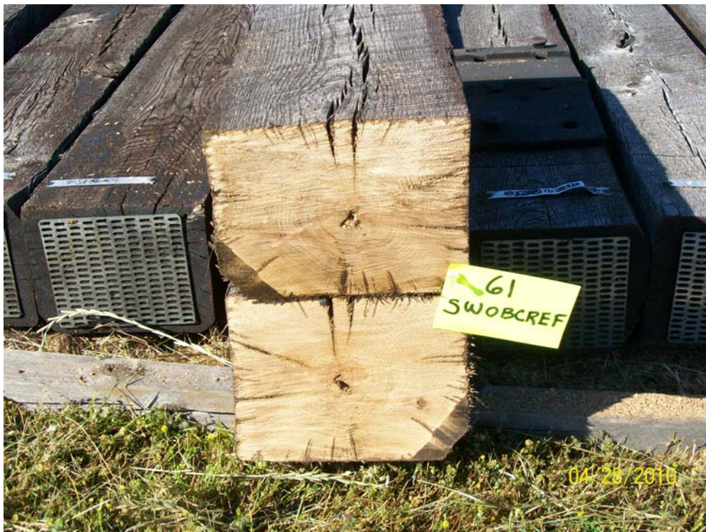
Figure 14 - Tie #61 (Boatright/white oak/borate/creosote to refusal).
