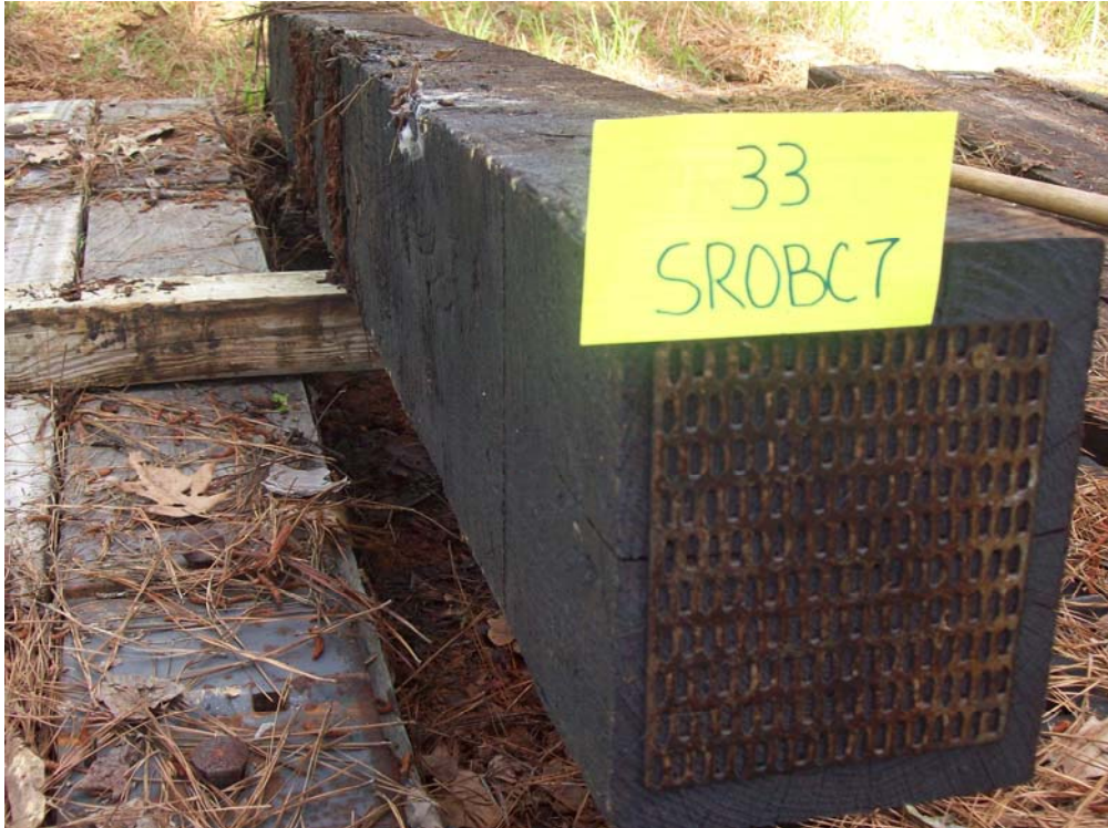
Figure 55 - Tie #33 (Boatright/red oak/borate/creosote 7pcf).
