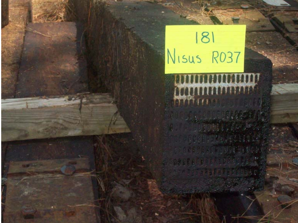
Figure 27- Tie #181 (Nisus/red oak/borate/oil A).
