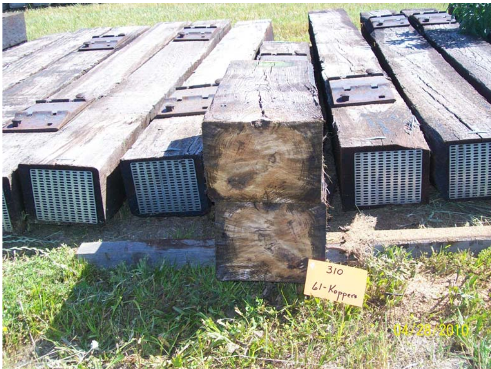
Figure 39 - Tie #310 (Koppers/white oak/creosote petroleum solution).
