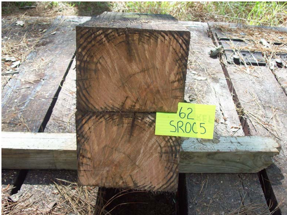
Figure 46 - Tie #62 (Boatright/red oak/creosote 5pcf).
