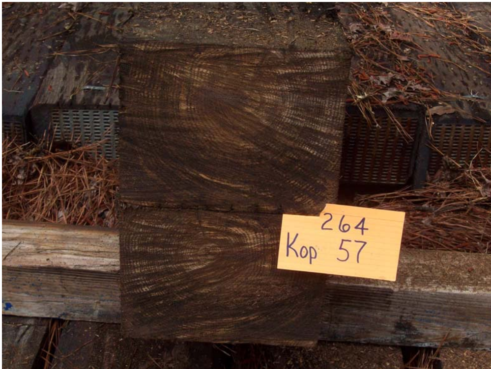
Figure 8 - Tie #264 card mislabeled – actually Kop 67 (Koppers/white oak/creosote petroleum).
