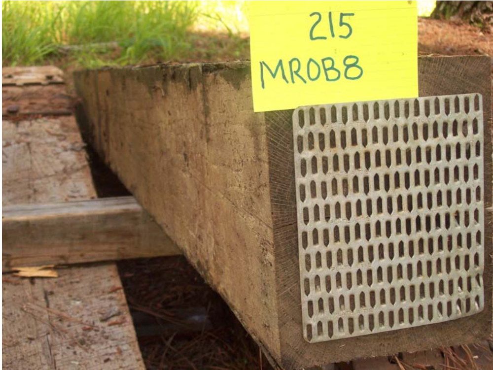
Figure 35 - Tie #215 (Merichem/red oak/borate/CuNap).
