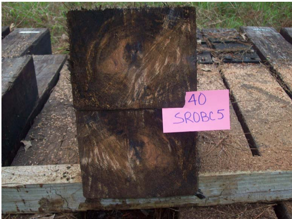
Figure 58 - Tie #40 (Boatright/red oak/borate/creosote 5pcf).
