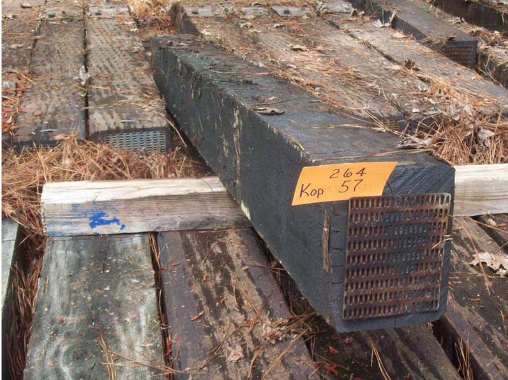
Figure 7 - Tie #264 card mislabeled – actually Kop 67 (Koppers/white oak/creosote petroleum).
