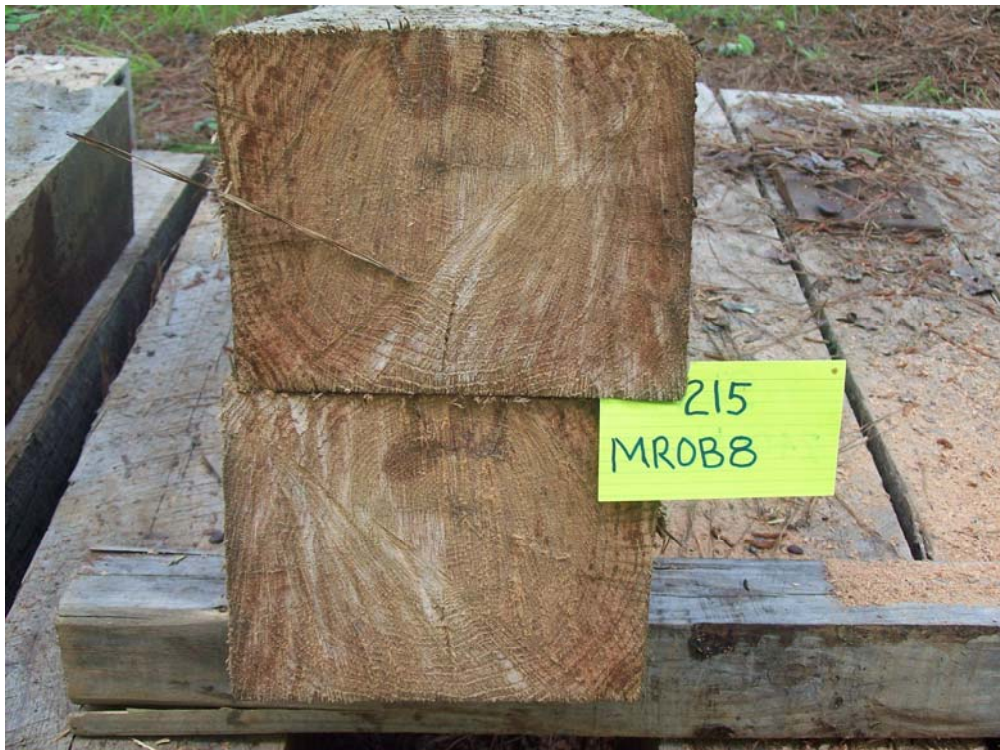
Figure 36 - Tie #215 (Merichem/red oak/borate/CuNap).
