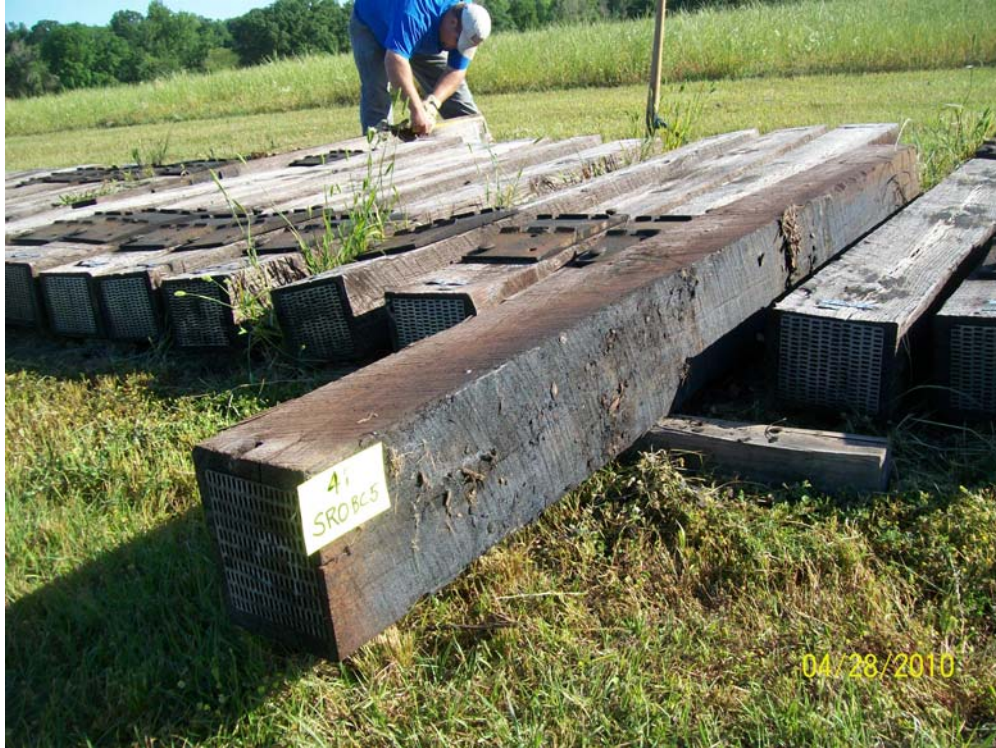
Figure 9 - Tie #41 (Boatright/red oak/borate/creosote 5pcf).
