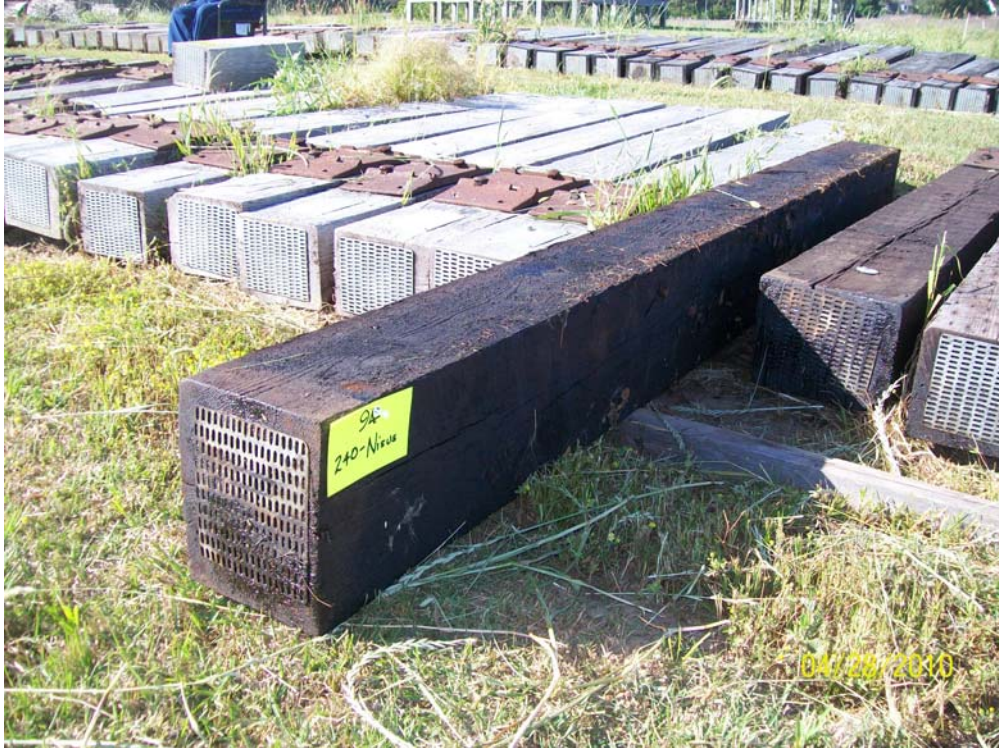
Figure 22 - Tie #94 (Nisus/red oak/borate/oil A).
