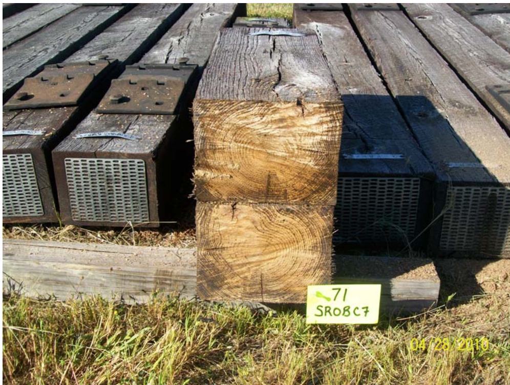
Figure 16 - Tie #71 (Boatright/red oak/borate/creosote 7pcf).
