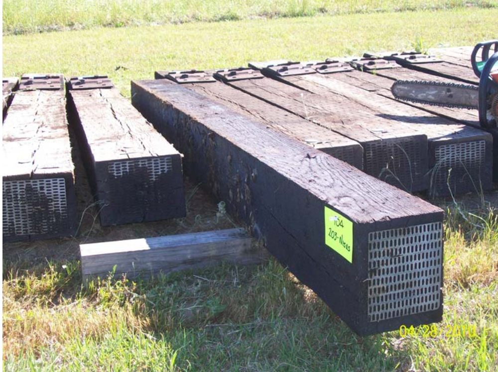
Figure 24 - Tie #104 (Nisus/red oak/borate/oil B).
