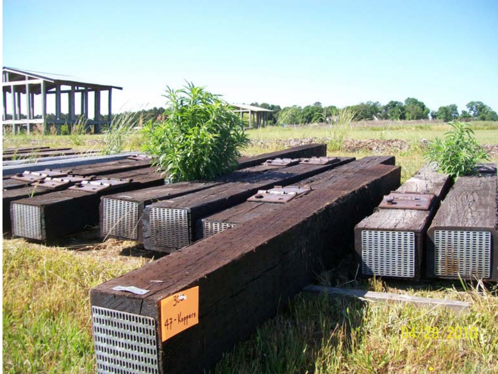
Figure 40 - Tie #300 (Koppers/red oak/creosote petroleum solution).
