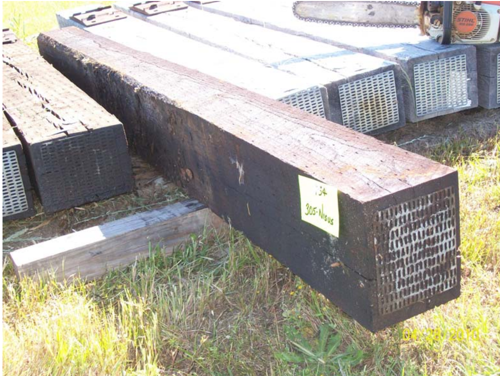
Figure 30 - Tie #134 (Nisus/white oak/borate/oil A).
