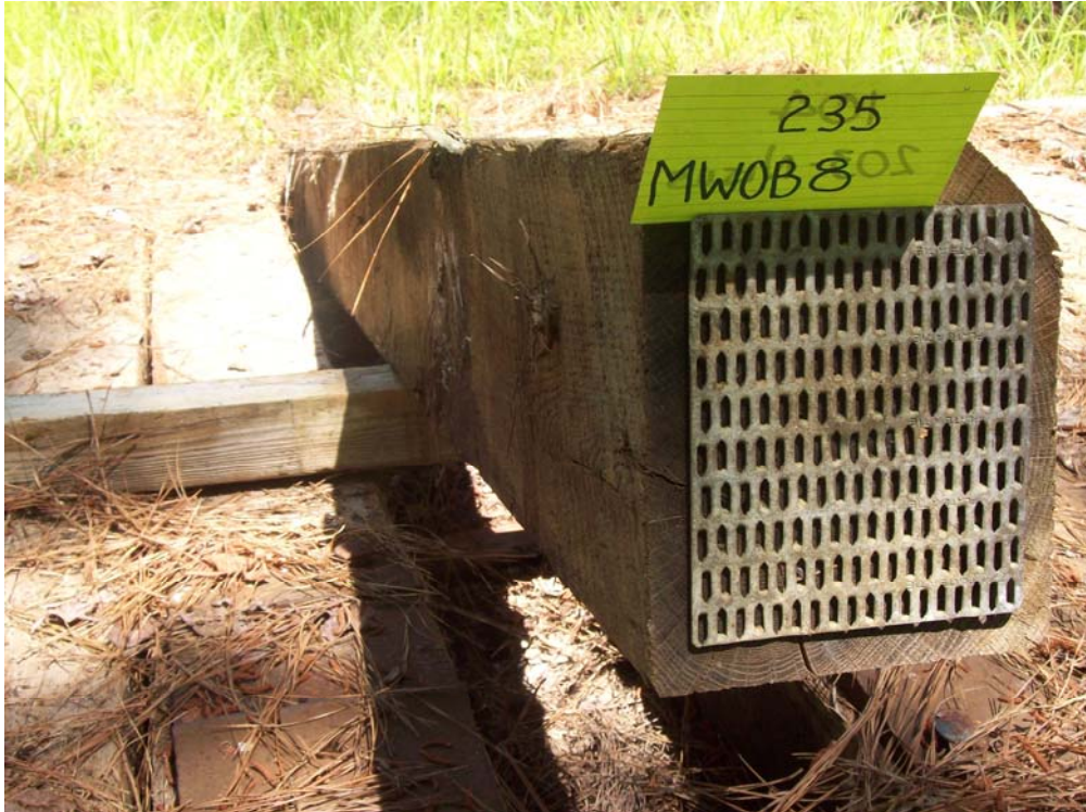
Figure 33 – Tie #235 (Merichem/white oak/borate/CuNap).
