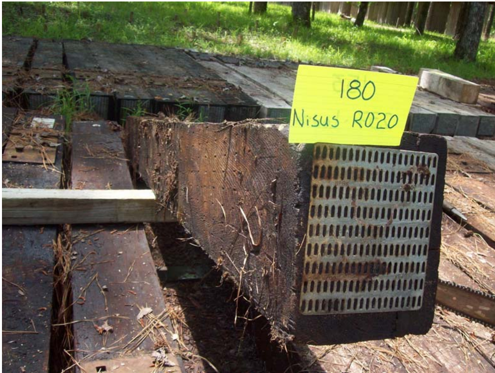
Figure 23- Tie #180 (Nisus/red oak/borate/oil B).
