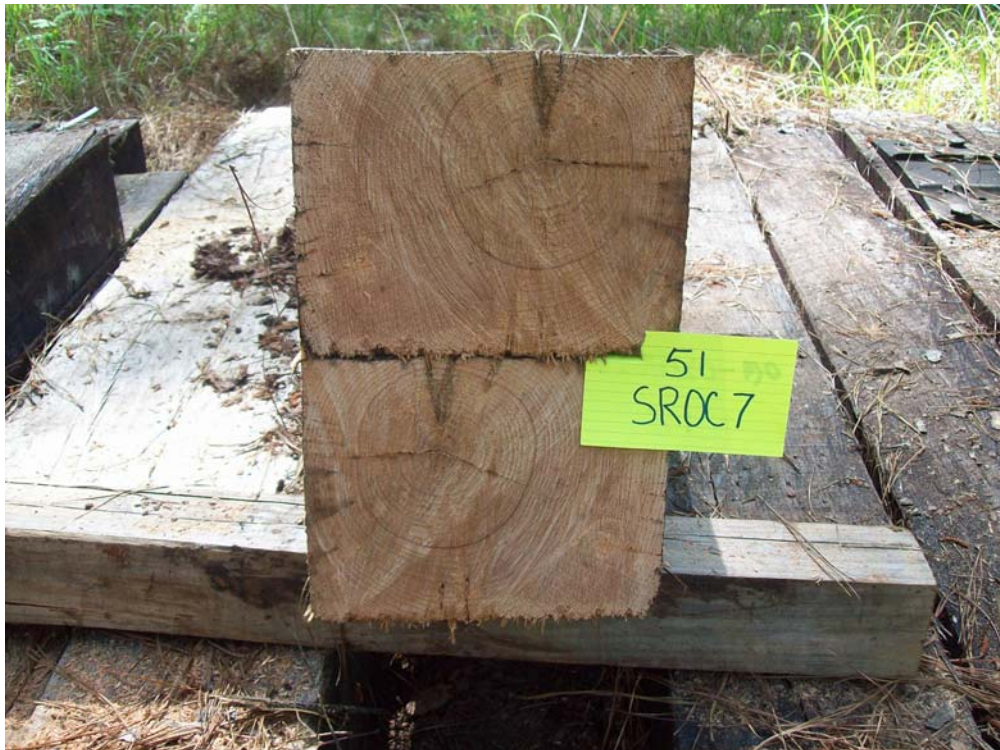
Figure 50 - Tie #51 (Boatright/red oak/untreated control).
