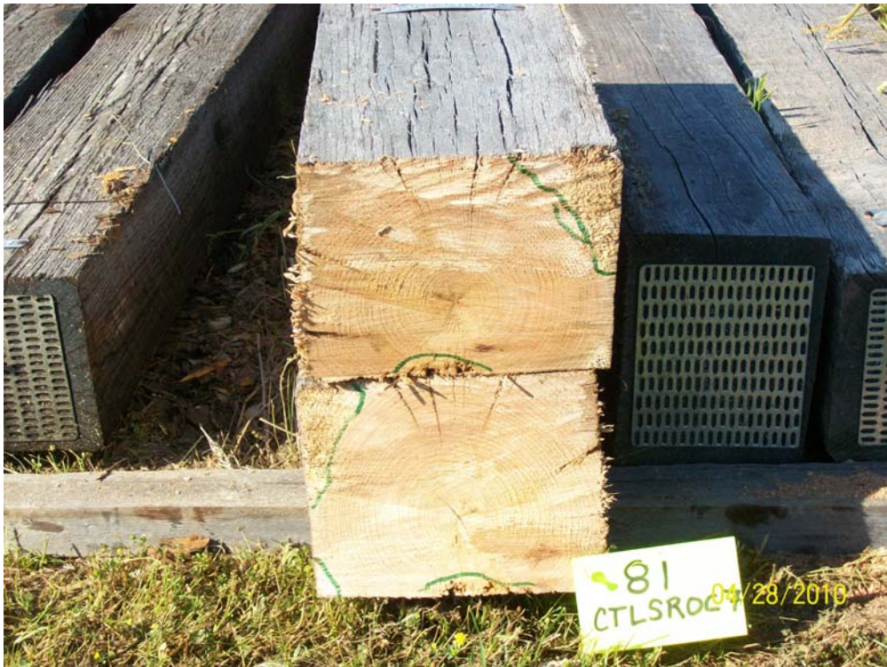
Figure 18 - Tie #81 (red oak/untreated) with decayed areas outlined.
