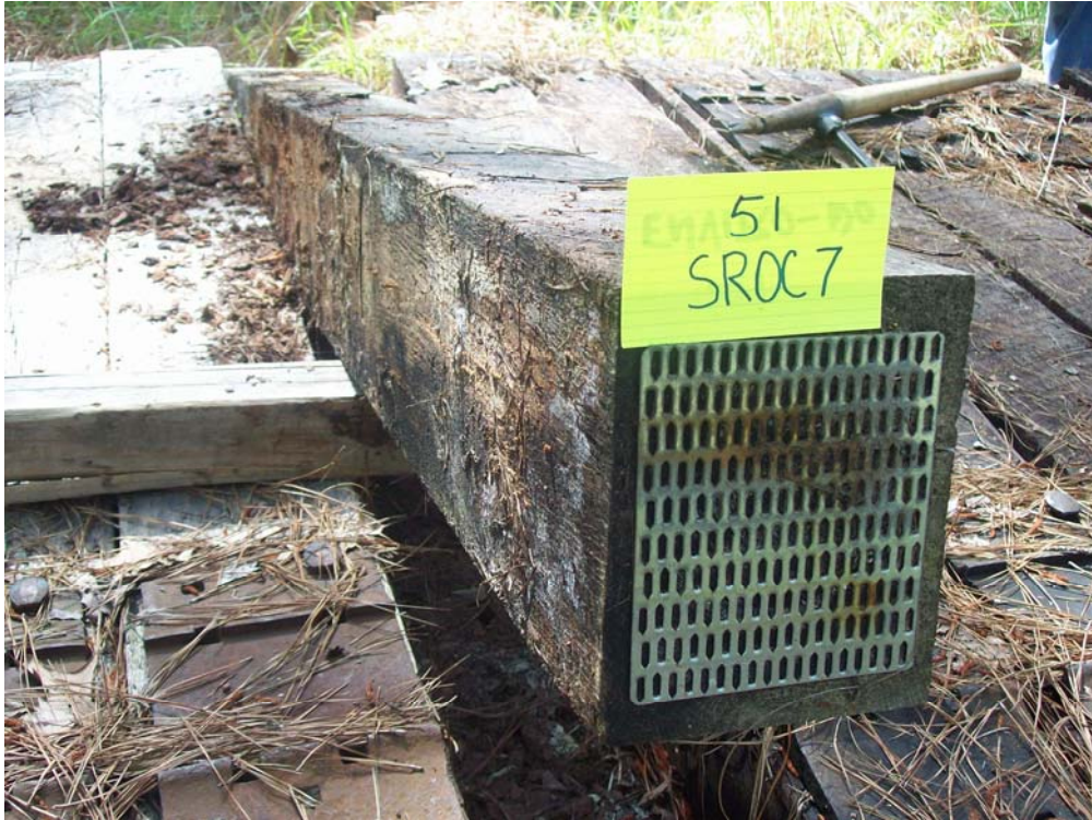
Figure 49 - Tie #51 (Boatright/red oak/untreated control).
