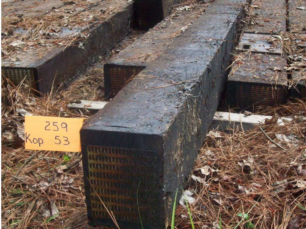
Figure 9 - Tie #259 (Koppers/red oak/creosote petroleum solution).
