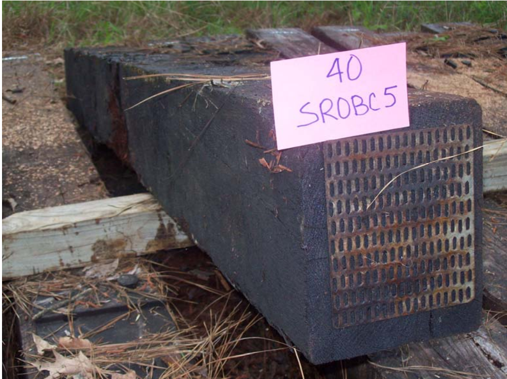
Figure 57 - Tie #40 (Boatright/red oak/borate/creosote 5pcf).
