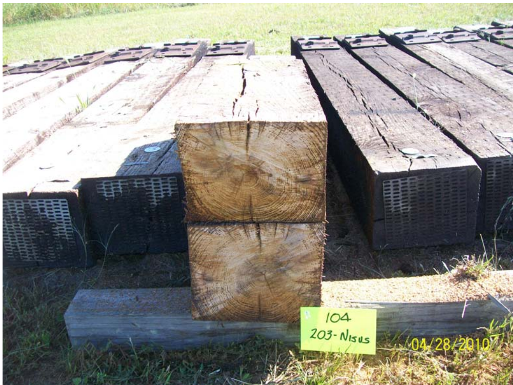
Figure 25 - Tie #104 (Nisus/red oak/borate/oil B).
