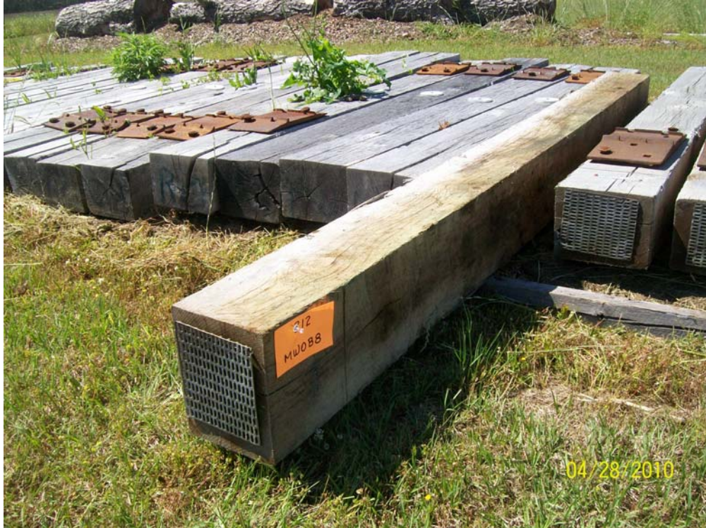
Figure 54 - Tie #212 (Merichem/white oak/borate/CuNap).
