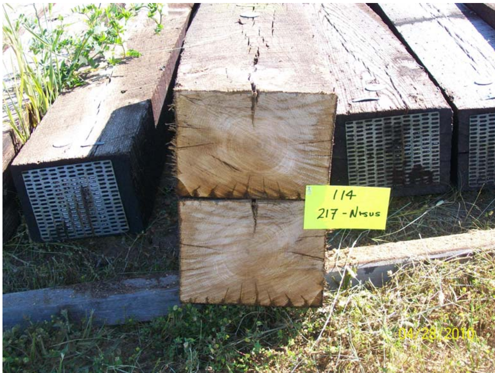
Figure 27 - Tie #114 (Nisus/white oak/borate/oil B).
