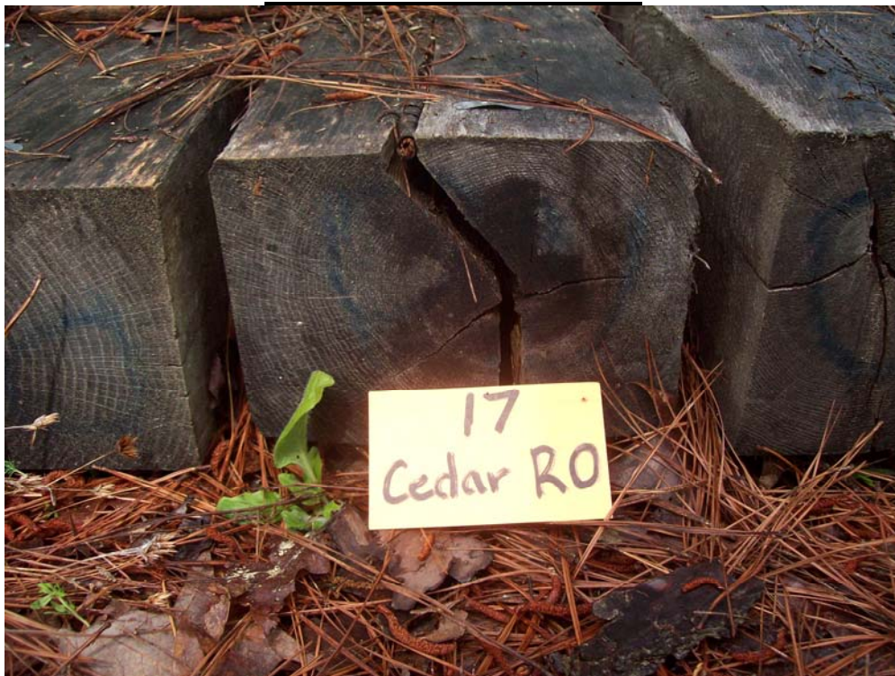
Figure 3 - Tie #17 (Cedarcide/red oak) showing splitting.
