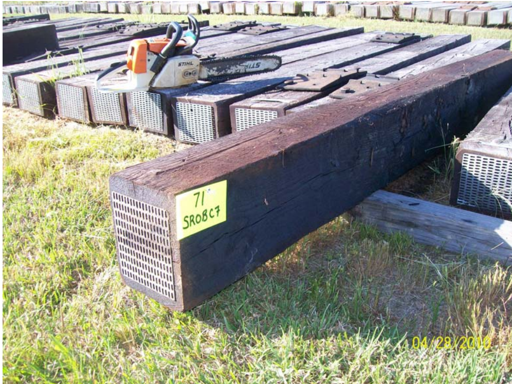
Figure 15 - Tie #71 (Boatright/red oak/borate/creosote 7pcf).
