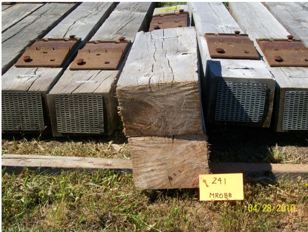
Figure 49 - Tie #241 (Merichem/red oak/borate/CuNap).
