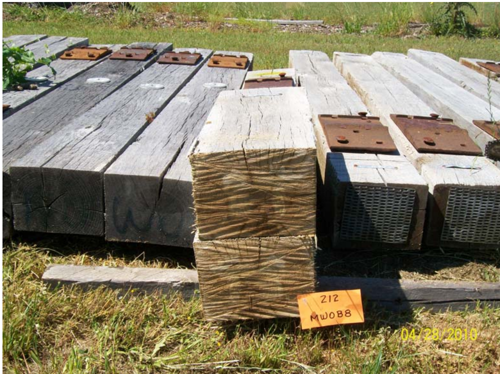
Figure 55 - Tie #212 (Merichem/white oak/borate/CuNap).
