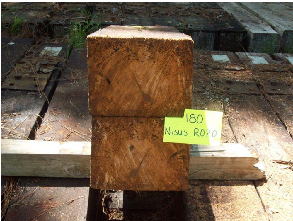
Figure 24 - Tie #180 (Nisus/red oak/borate/oil B).
