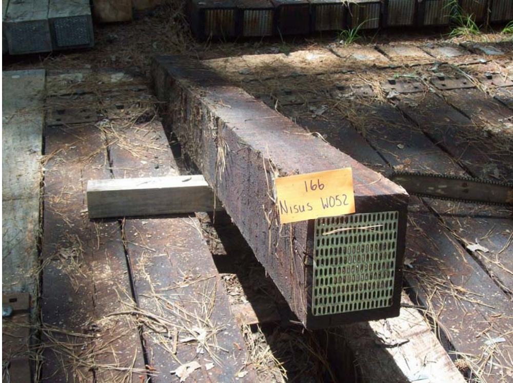
Figure 19- Tie#166 (Nisus/white oak/borate/oil B).
