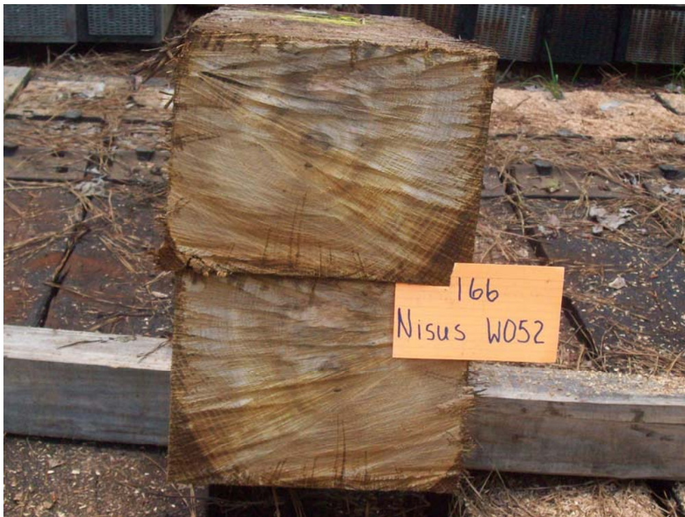
Figure 20 - Tie#166 (Nisus/white oak/borate/oil B).
