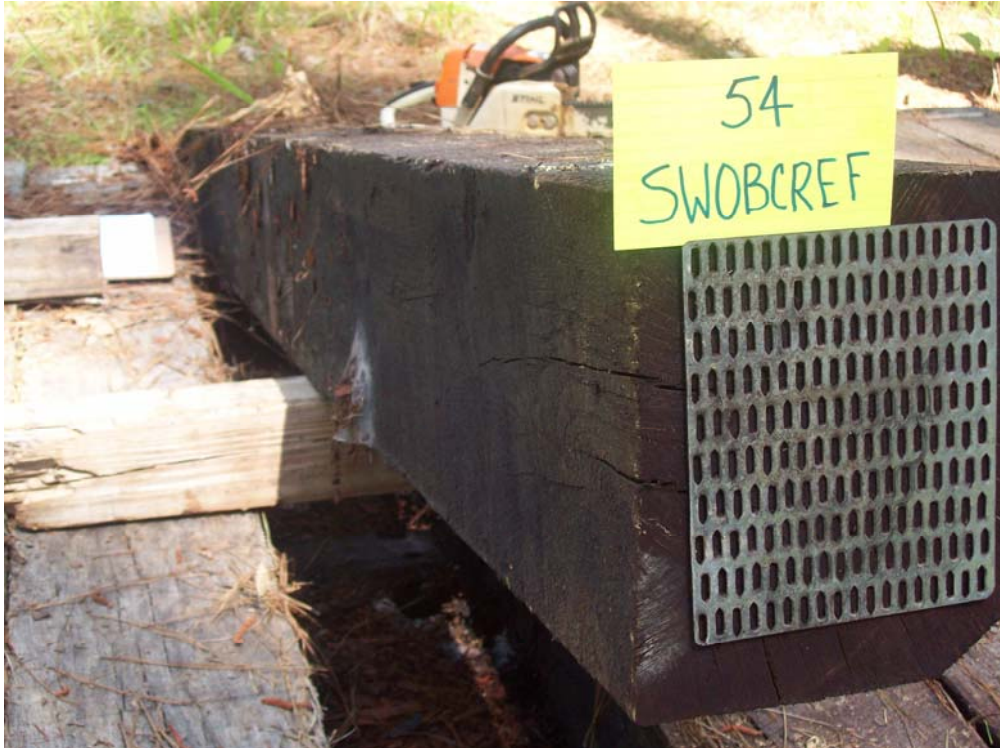
Figure 47 Tie #54 (Boatright/white oak/borate/creosote to refusal).
