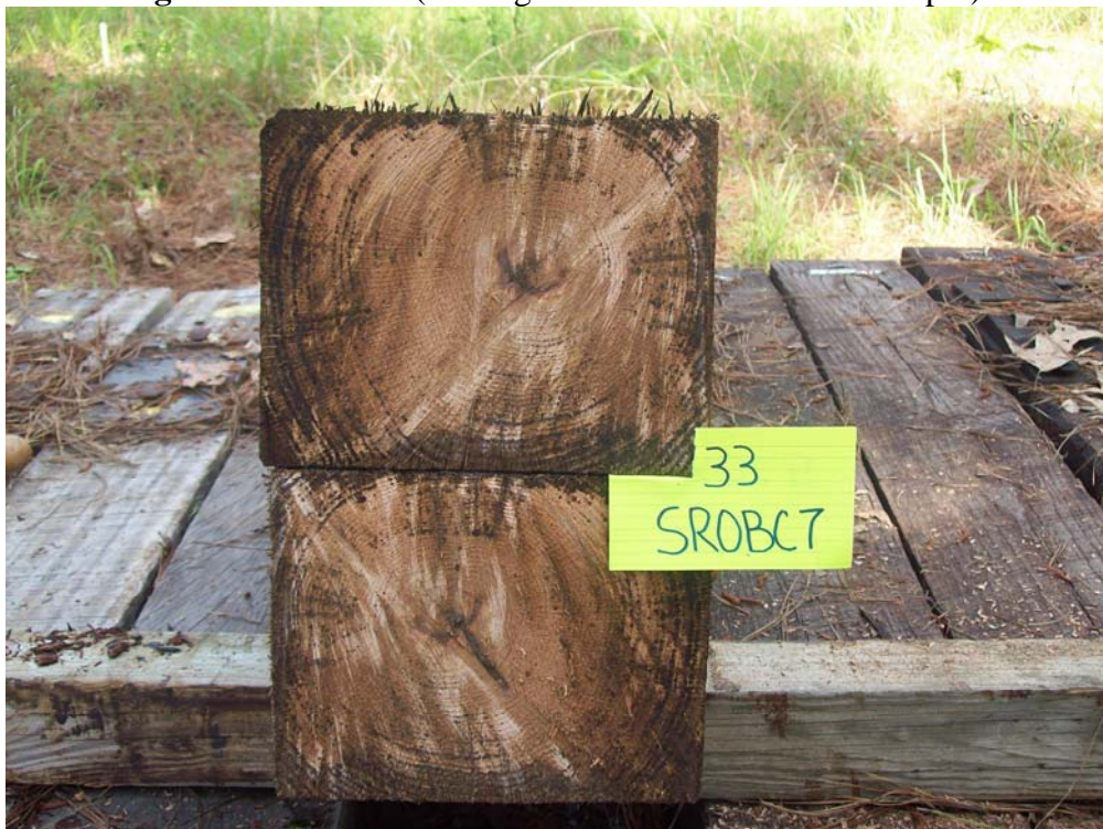
Figure 56 - Tie #33 (Boatright/red oak/borate/creosote 7pcf).
