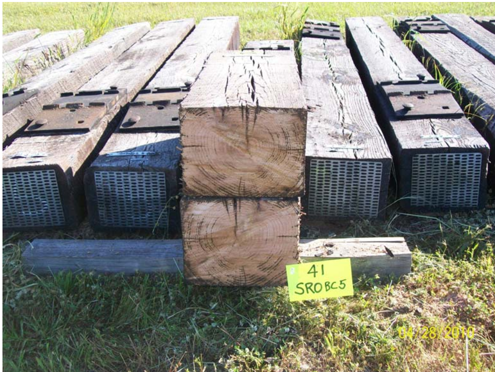
Figure 10 - Tie #41 (Boatright/red oak/borate/creosote 5pcf).
