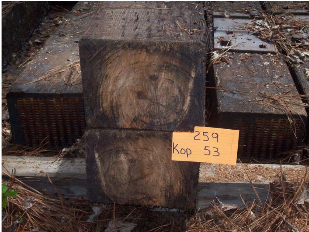
Figure 10 - Tie #259 (Koppers/red oak/creosote petroleum solution).
