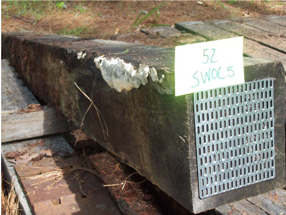
Figure 51 Tie #52 (Boatright/white oak/untreated control).
