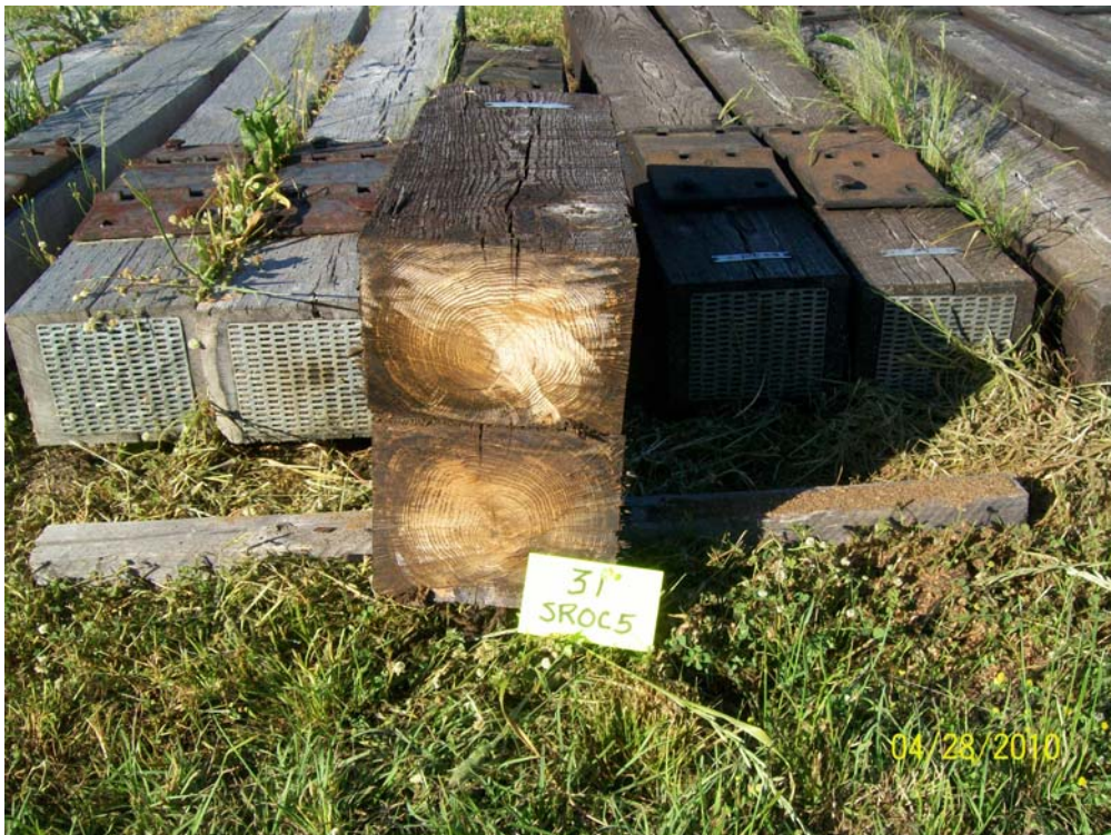
Figure 8 – Tie #31 (Boatright/red oak/creosote 5pcf).
