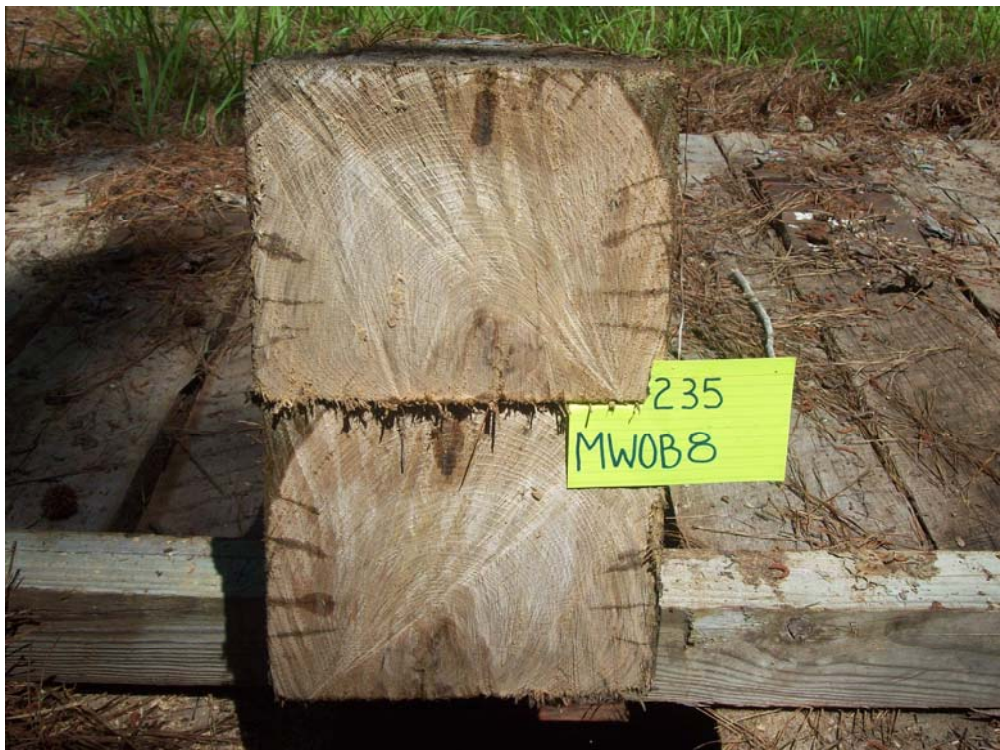
Figure 34 – Tie #235 (Merichem/white oak/borate/CuNap).
