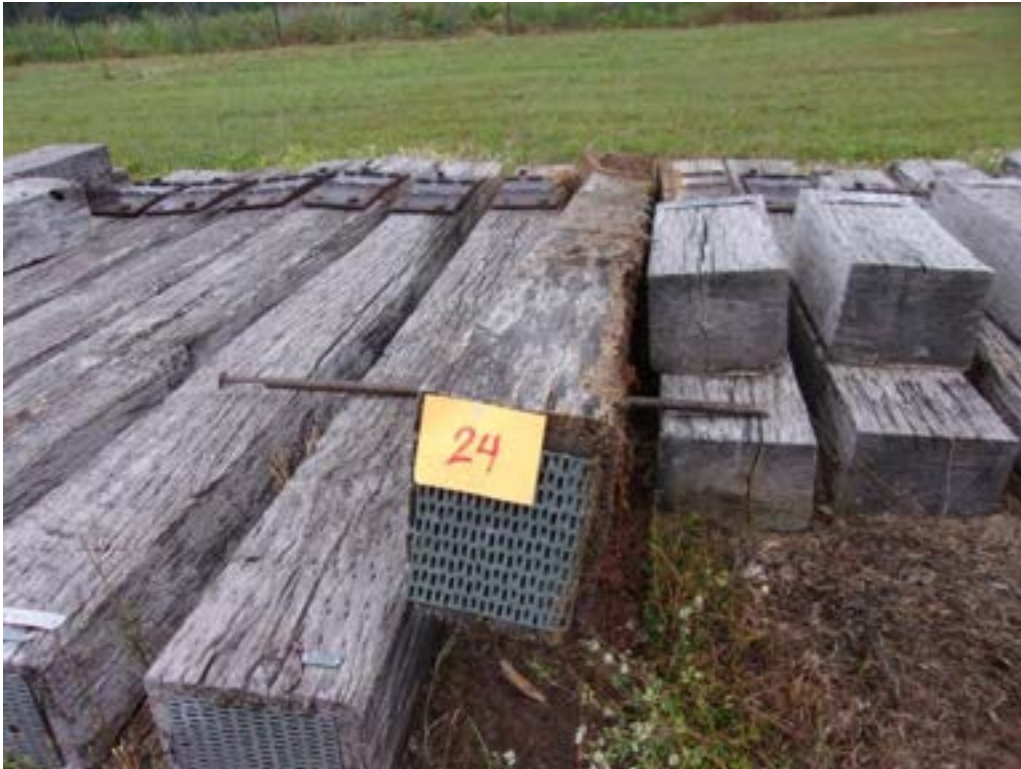
A69 – Tie #24 (Envirosafe/white oak) with on side & bottom.
