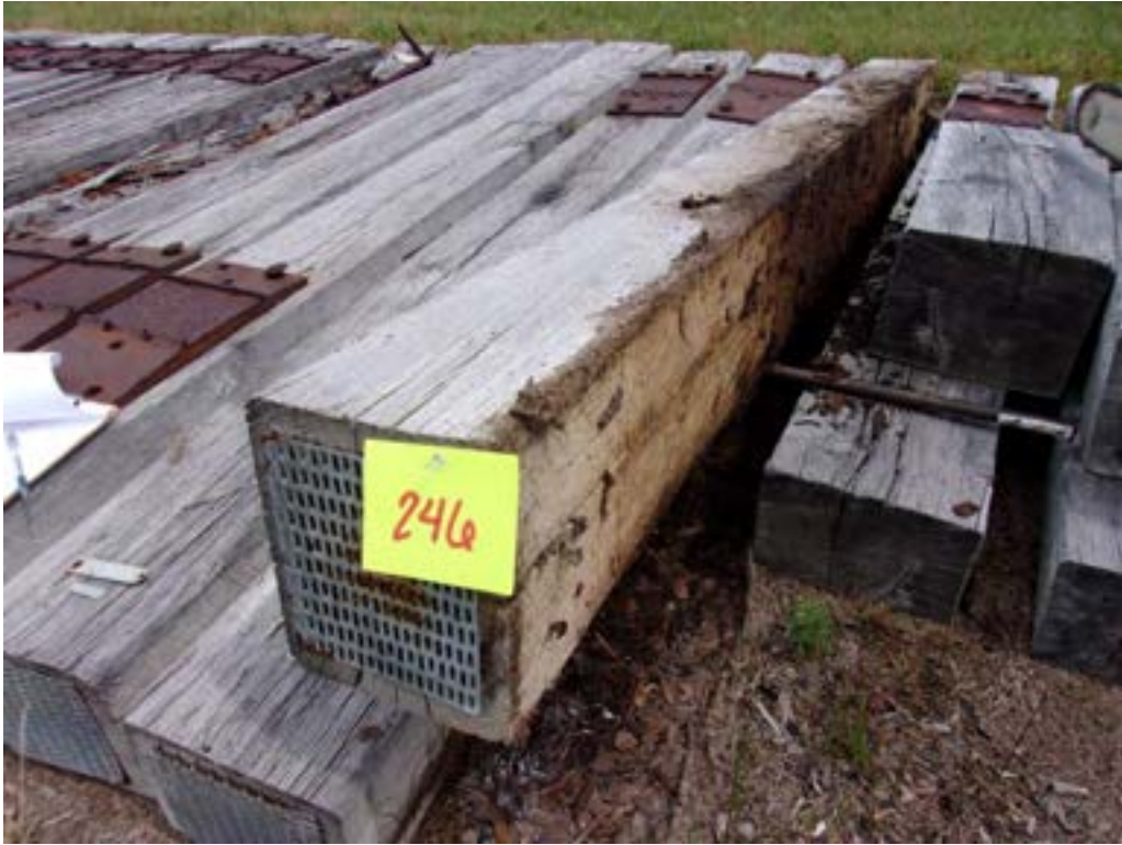
A115 - Tie #246 (Merichem/red oak/borate/CuNap) with trace termite damage.
