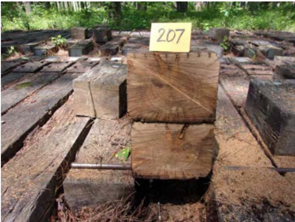
A42 - Tie #207 (Nisus/white oak/borate) with decay near checks & on bottom.
