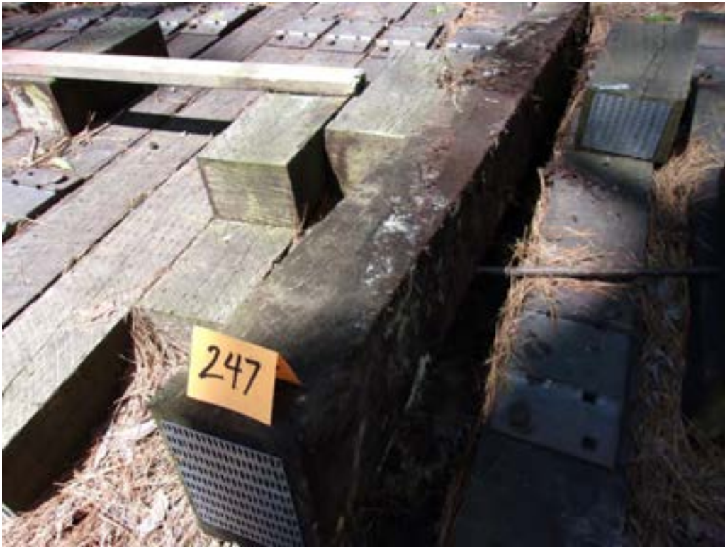
A51 - Tie #247 (Koppers/white oak/creosote petroleum solution).
