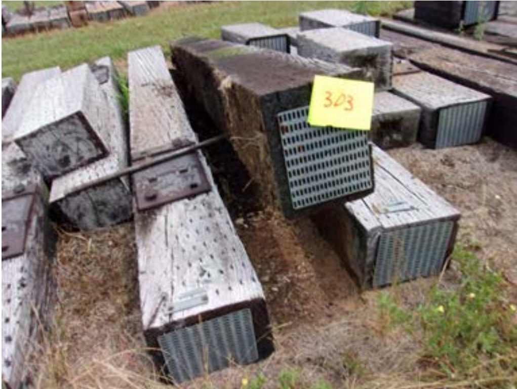
A123 - Tie #303 (Koppers/red oak/creosote petroleum solution).
