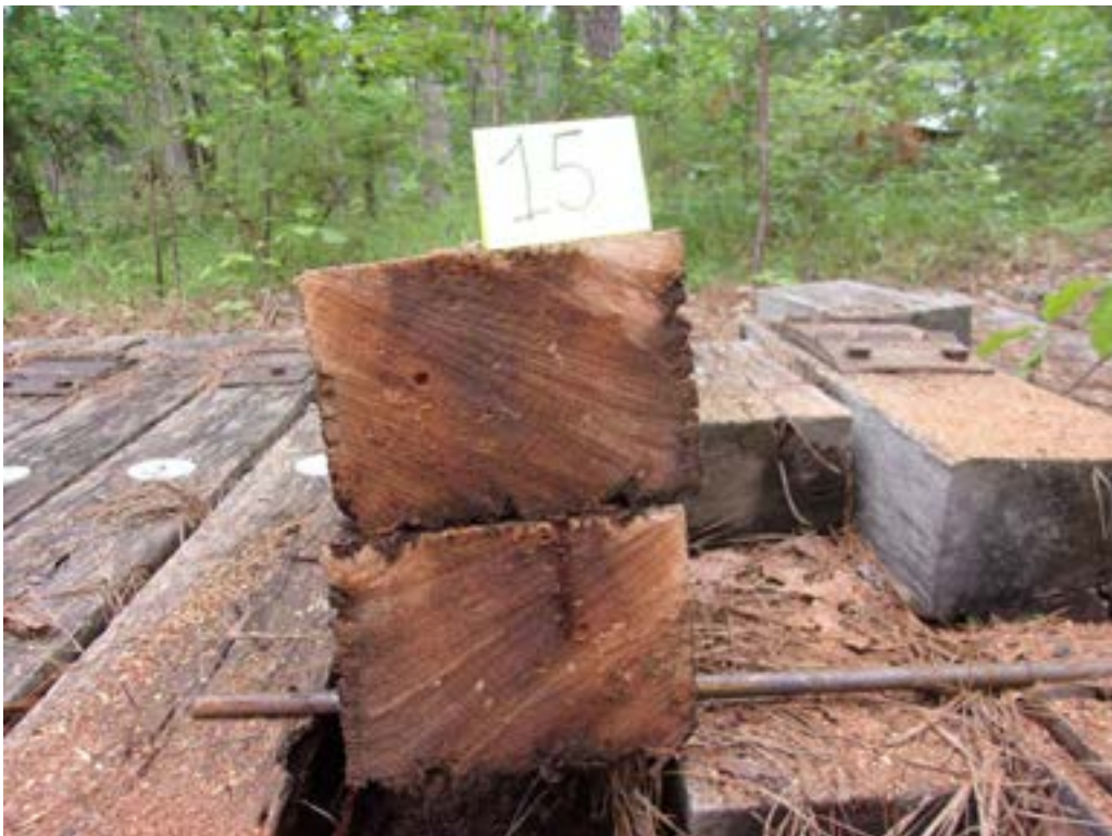
A4 – Tie #15 (Cedarcide/red oak) with decay.
