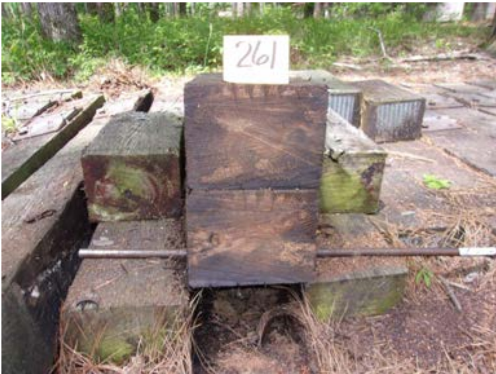
A54 - Tie #261 (Koppers/red oak/creosote petroleum solution).
