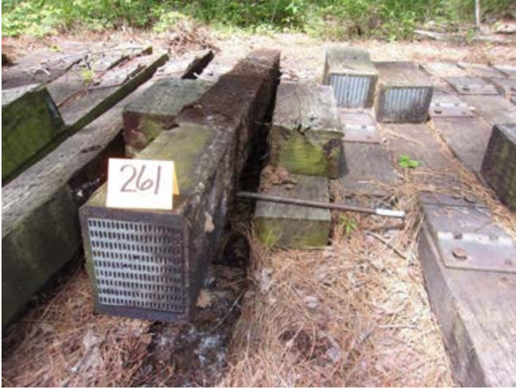
A53 - Tie #261 (Koppers/red oak/creosote petroleum solution).
