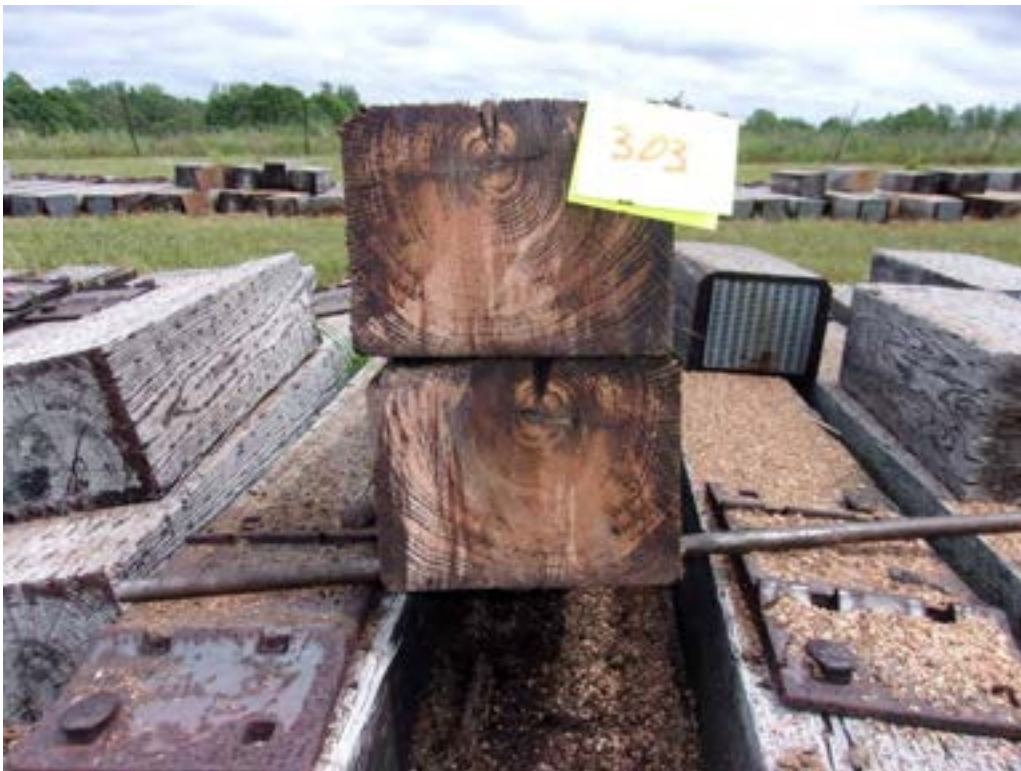
A124 - Tie #303 (Koppers/red oak/creosote petroleum solution).
