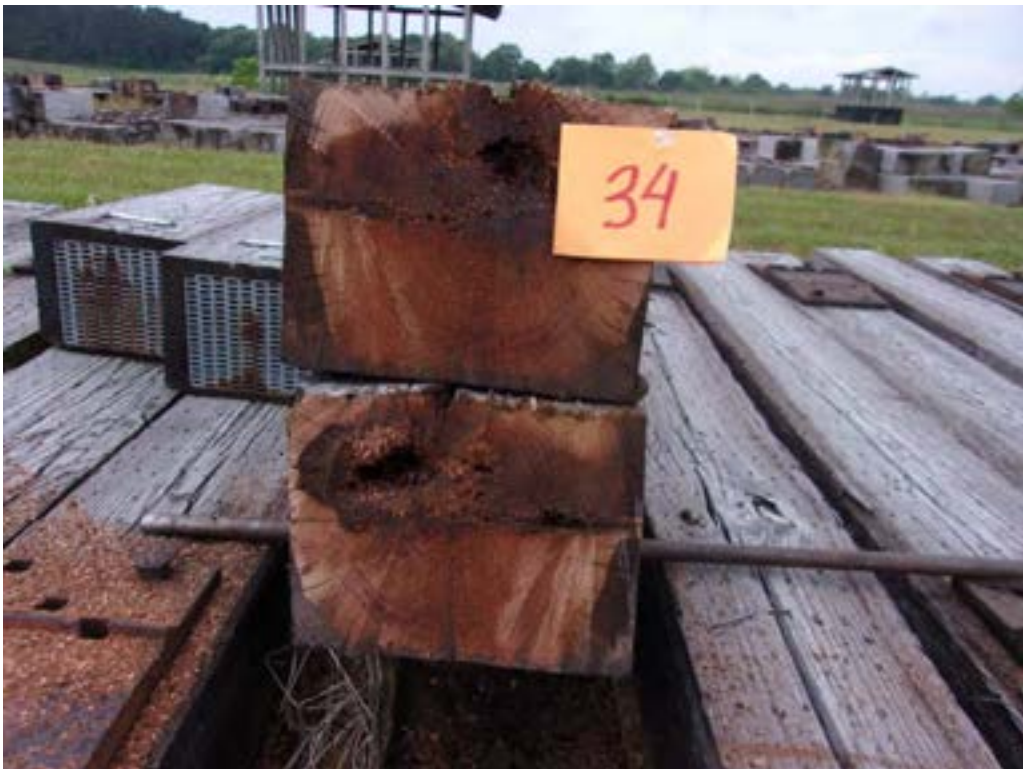
A72 – Tie #34 (Boatright/red oak/creosote 5pcf) internal decay around check.
