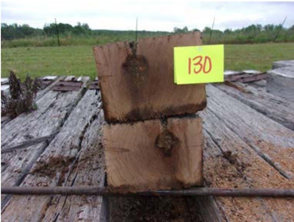
A90 - Tie #130 (Nisus/red oak/borate) with internal decay.
