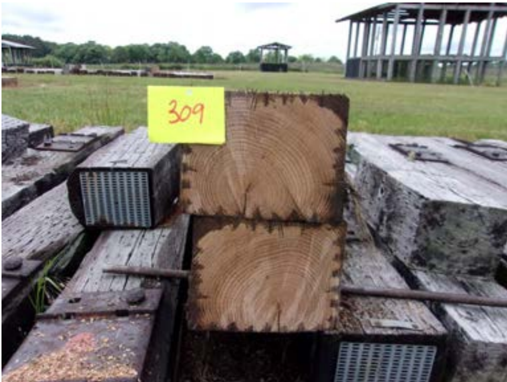
A126 - Tie #309 (Koppers/white oak/creosote petroleum solution).
