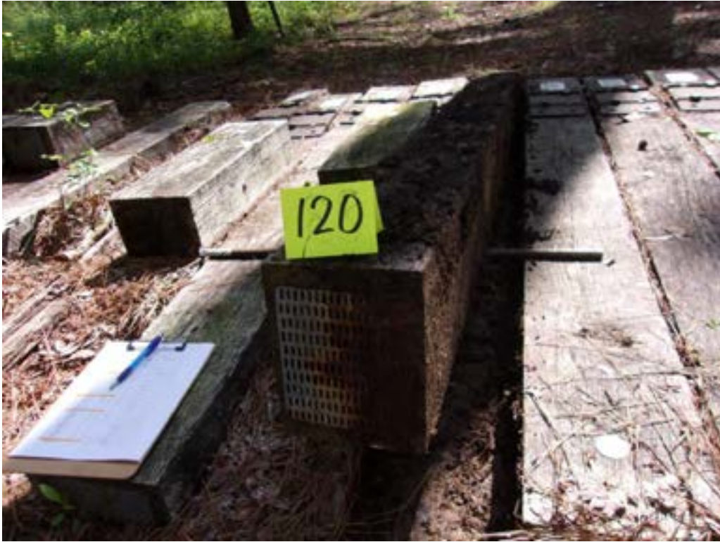
A23 - Tie #120 (Lonza/red oak) with decay & trace termite damage on bottom.
