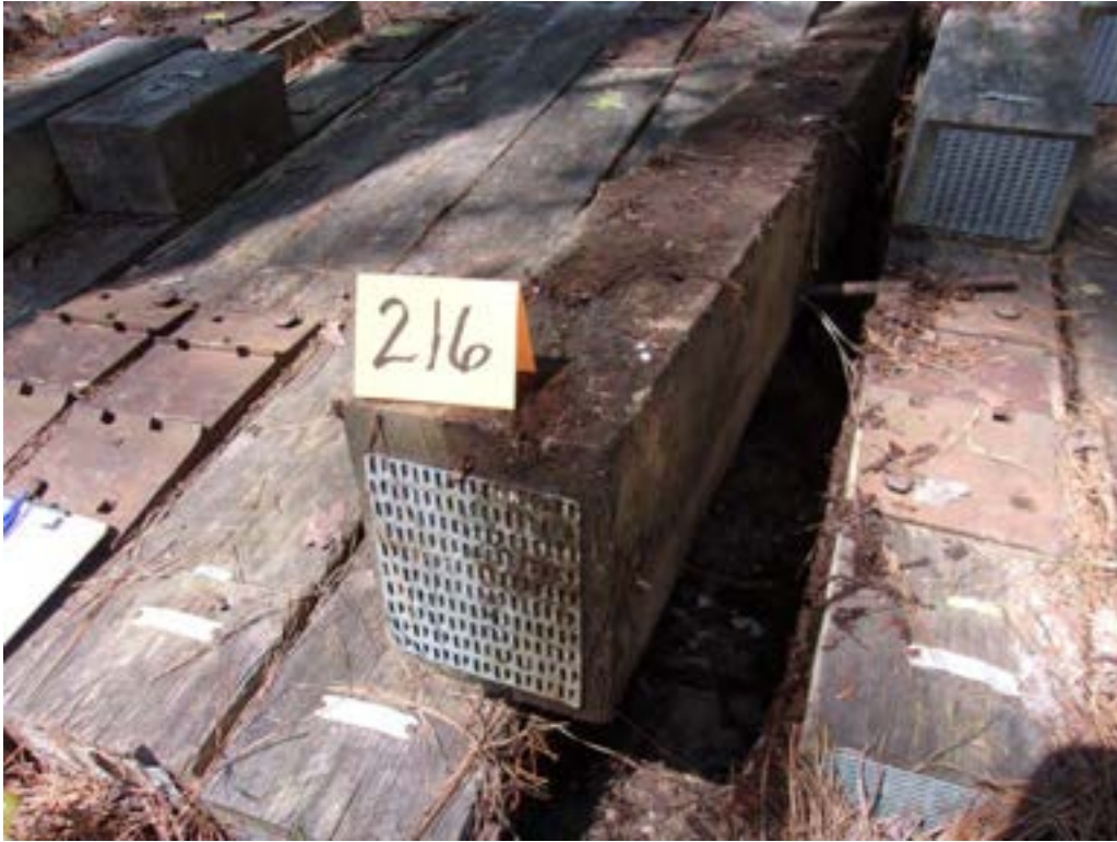
A43 - Tie #216 (Merichem/red oak/borate/CuNap) with trace decay.
