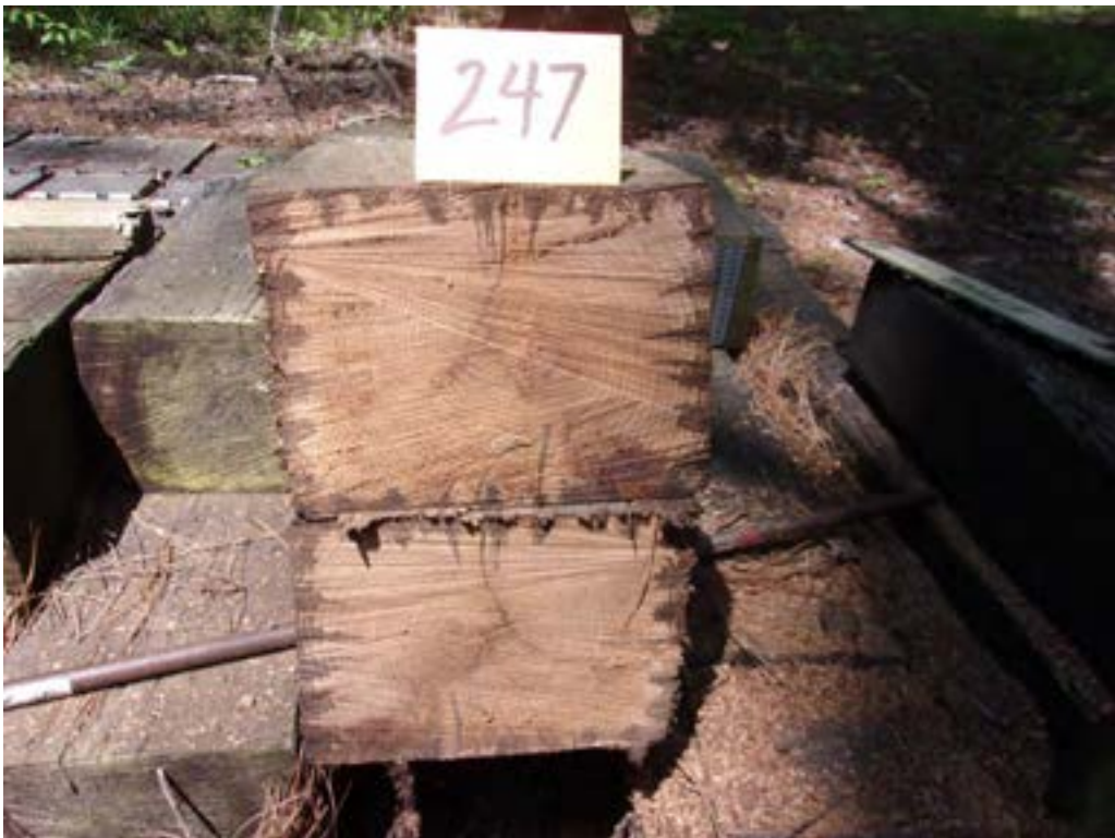
A52 - Tie #247 (Koppers/white oak/creosote petroleum solution).
