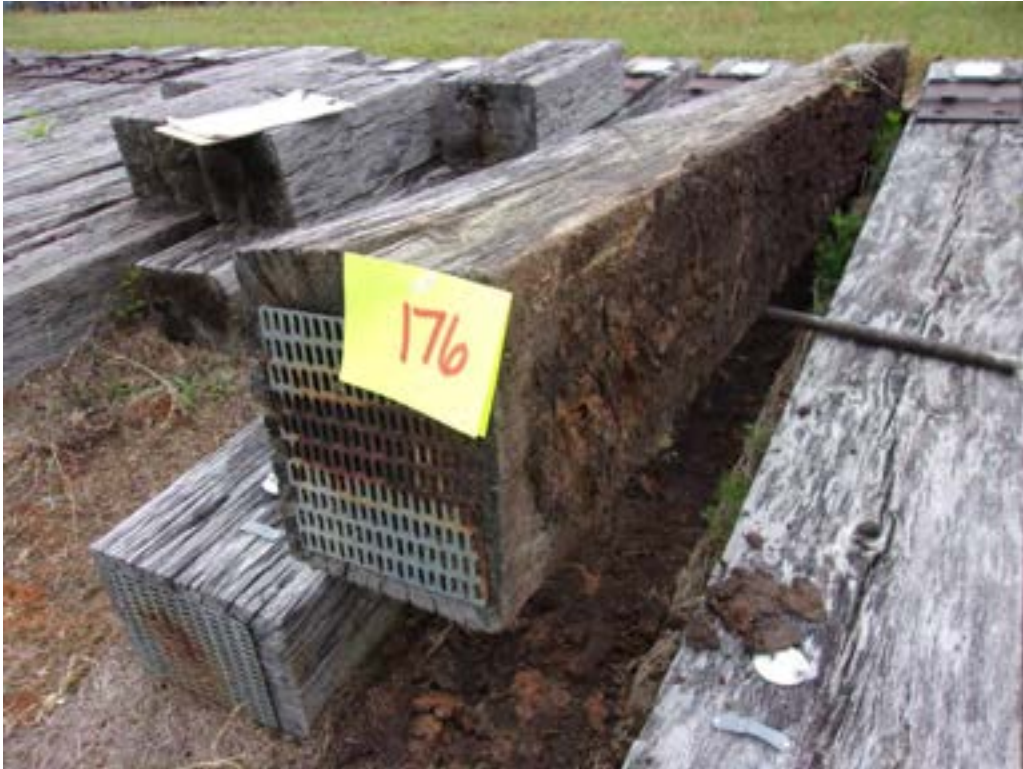
A103 – Tie #176 (Lonza/red oak) with decay and termite damage.
