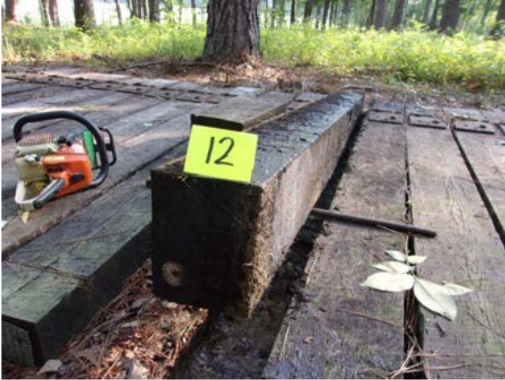
Figure 3 - Tie #12 red oak/borate/creosote 7lbs (Koppers).
