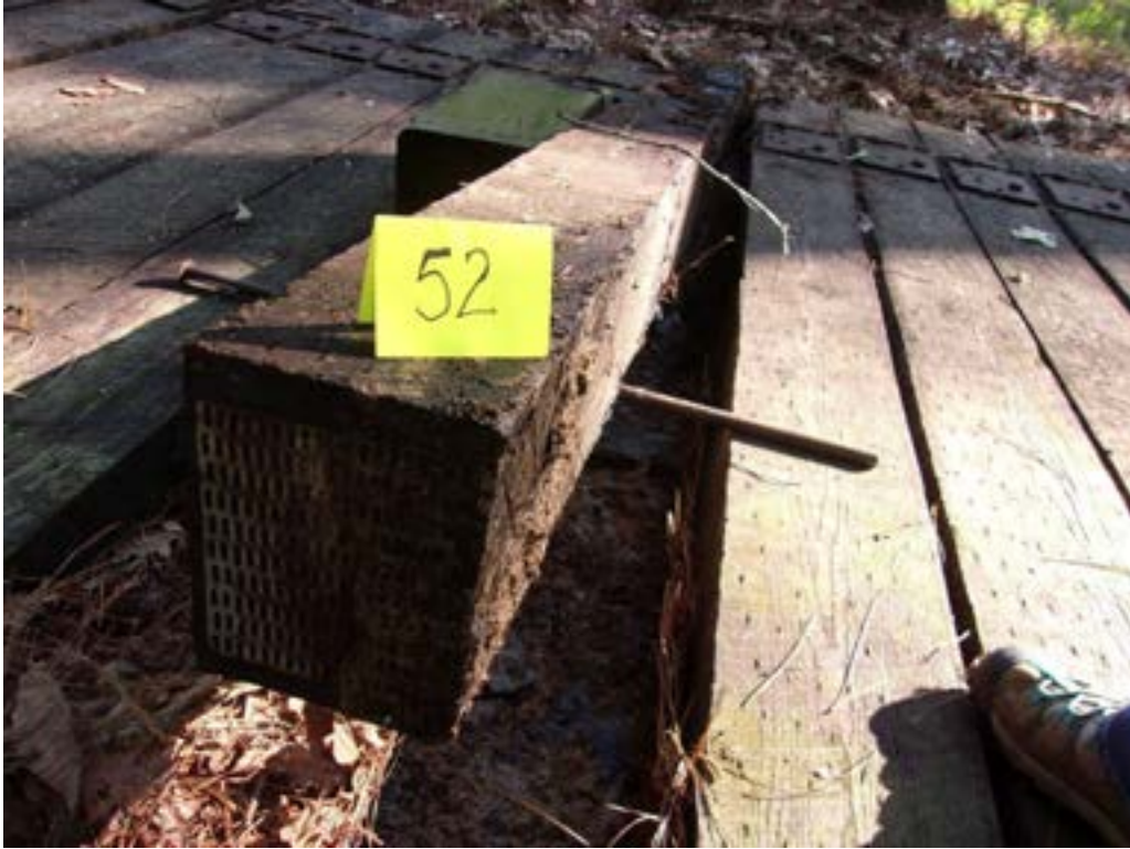
Figure 11 - Tie #52 red oak/borate/creosote 6lbs (Koppers).
