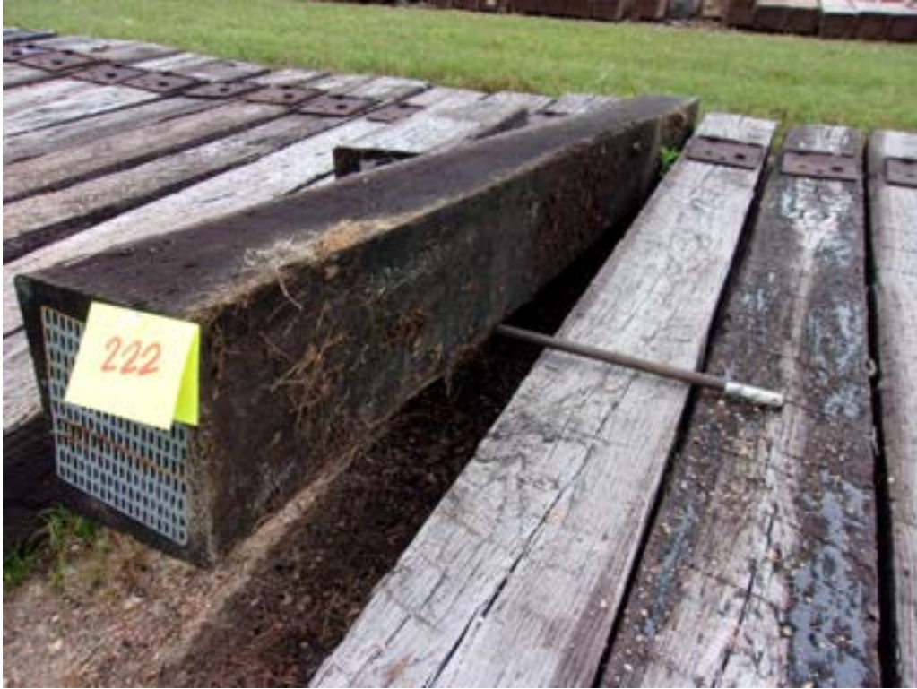
Figure 99 – Tie #222 red oak/borate/creosote 6lbs (Koppers).
