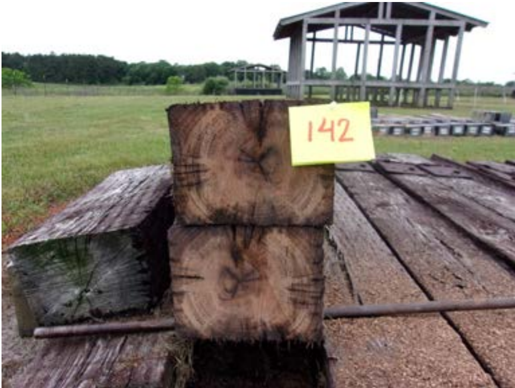
Figure 82 – Tie #142 red oak/DOT/ACZA/oil (Lonza).
