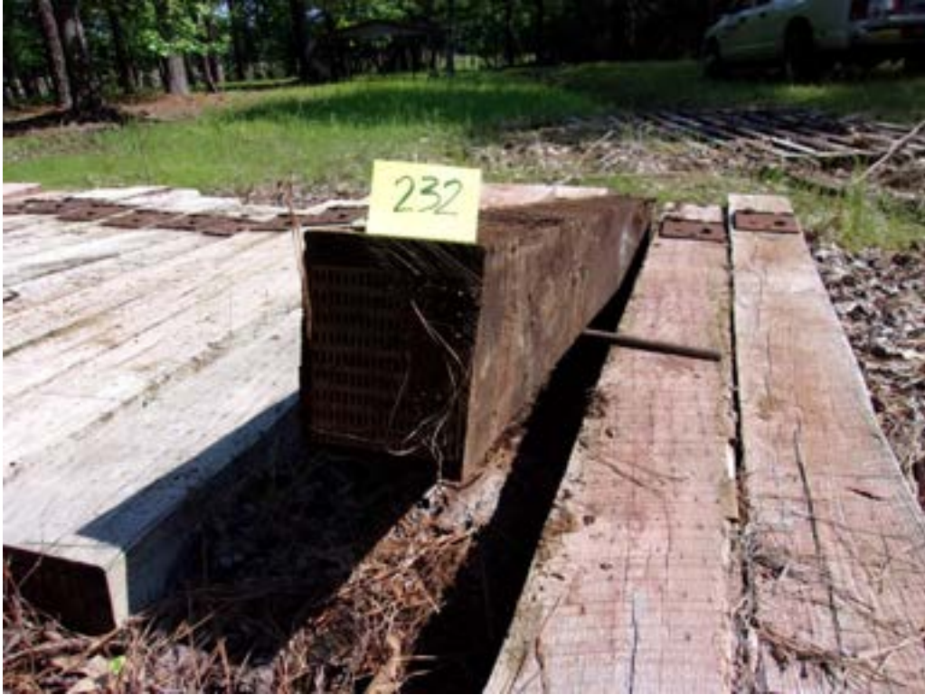
Figure 49 – Tie # 232 white oak/DOT/ACZA/ET (Lonza).
