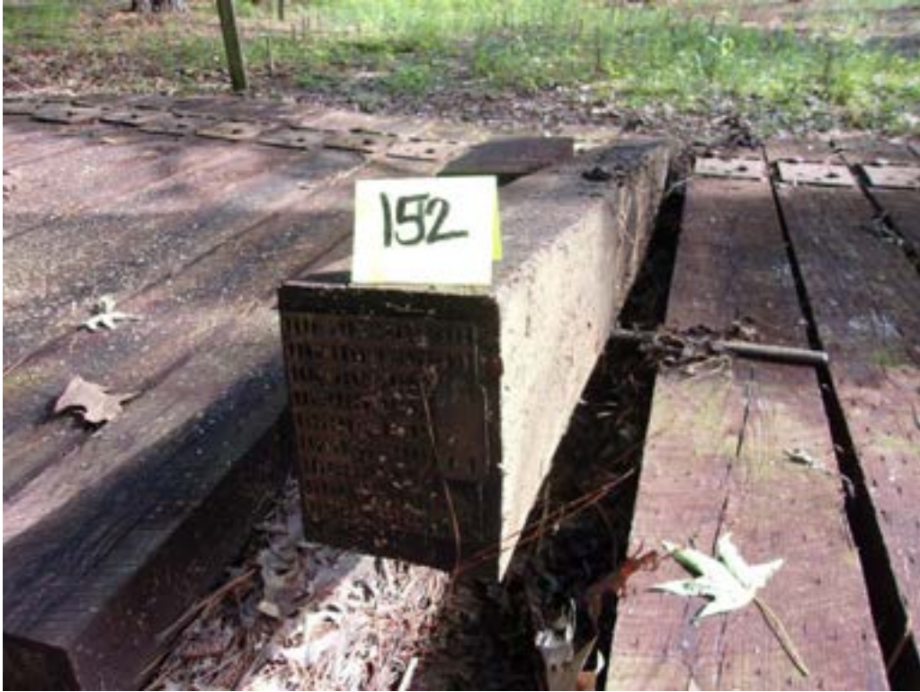
Figure 33 - Tie # 152 red oak/DOT/ACZA/oil (Lonza).
