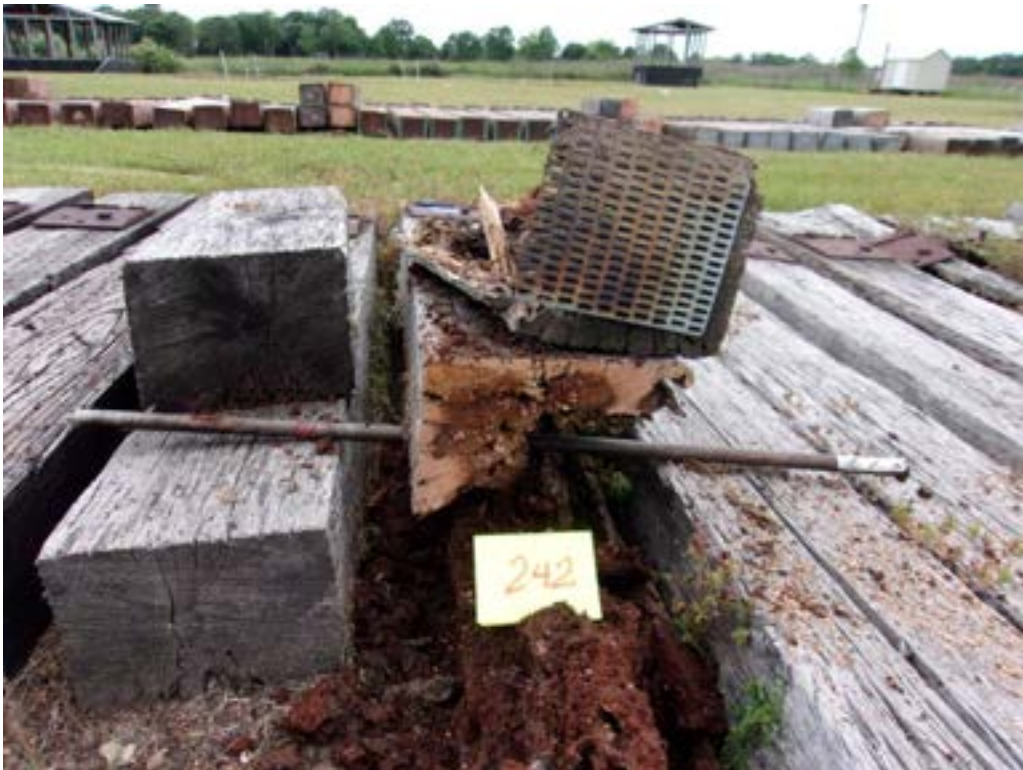
Figure 104 - Tie #242 untreated red oak with heavy decay and termite damage.
