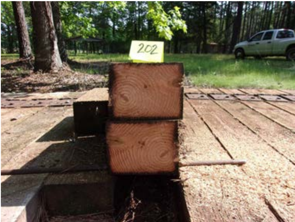
Figure 44 - Tie #202 Douglas fir/ACZA/DOT/ET (Lonza).
