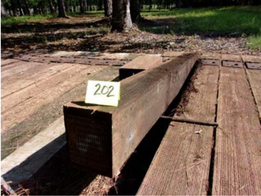
Figure 43 – Tie #202 Douglas fir/ACZA/DOT/ET (Lonza).
