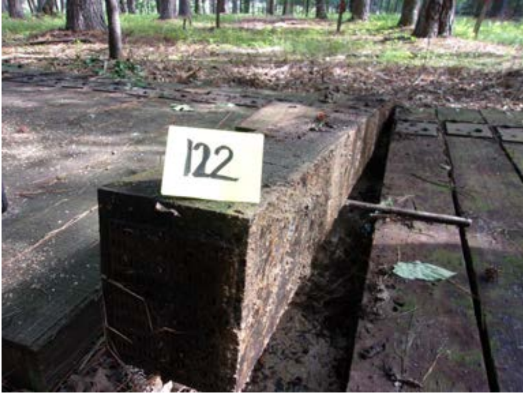
Figure 25 – Tie #122 red oak/DOT/ACZA/oil (Lonza).
