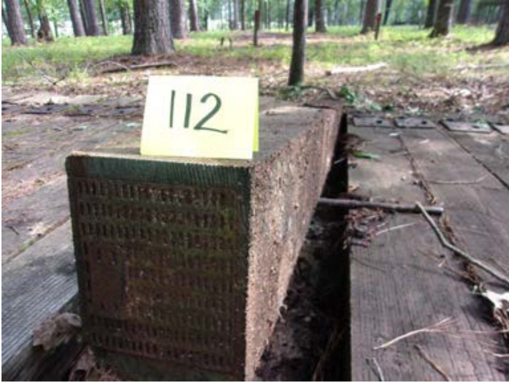
Figure 23 – Tie #112 Douglas fir/DOT/ACZA (Lonza).
