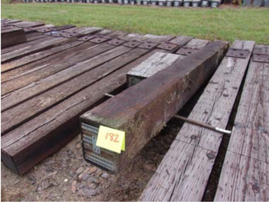
Figure 91 – Tie #182 Douglas fir/P2 (Lonza).
