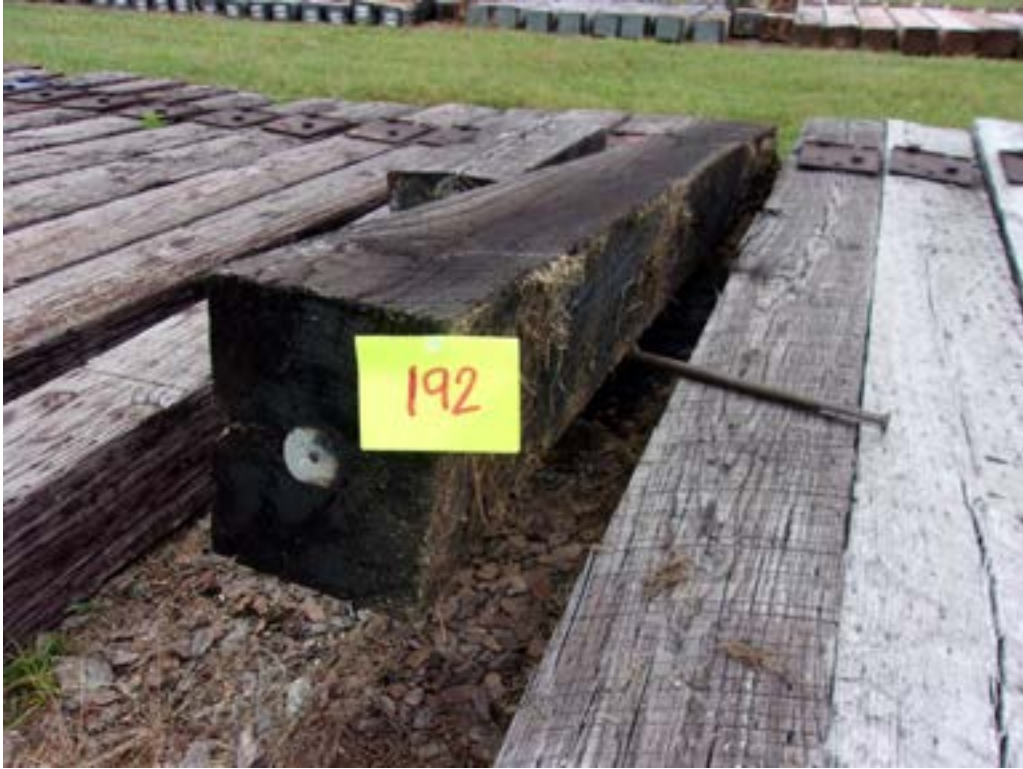
Figure 93 – Tie #192 white oak/borate/creosote/6lbs (Koppers).
