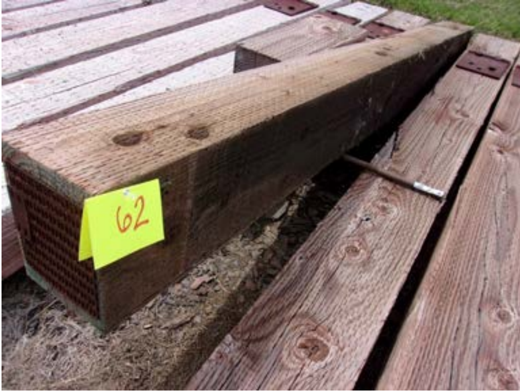
Figure 65 – Tie #62 Douglas fir/DOT/ACZA/ET (Lonza).
