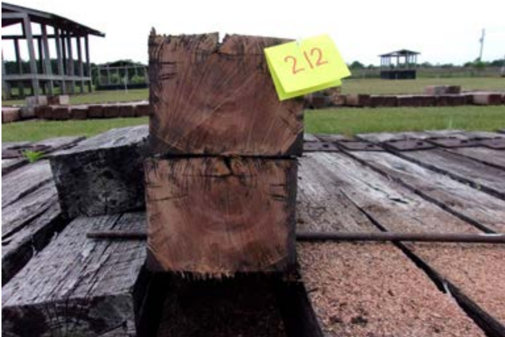
Figure 98 - Tie #212 red oak/borate/creosote 7lbs (Koppers).
