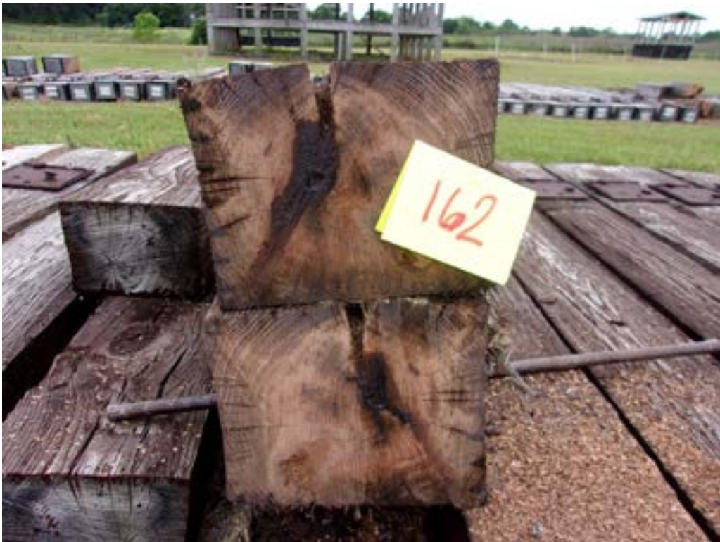
Figure 88 - Tie #162 red oak/DOT/ACZA/oil (Lonza).
