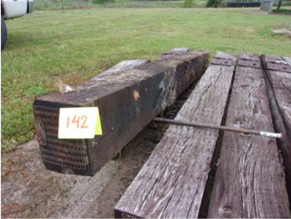
Figure 81 – Tie #142 red oak/DOT/ACZA/oil (Lonza).
