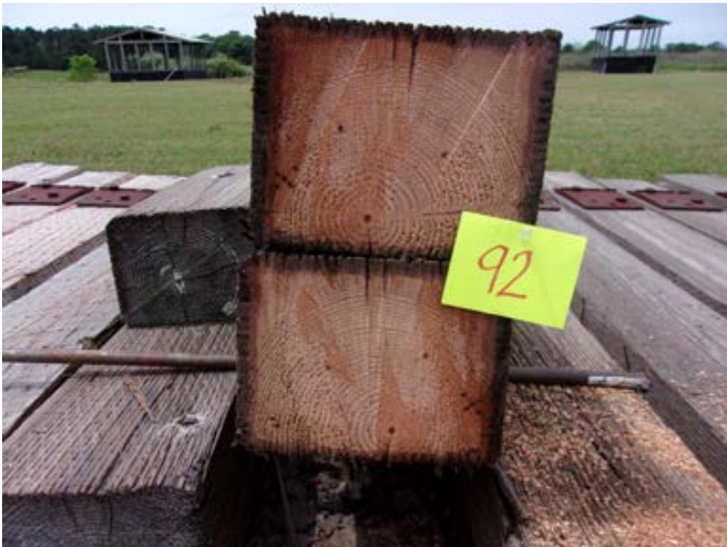
Figure 72 - Tie #92 Douglas fir/DOT/ACZA (Lonza).
