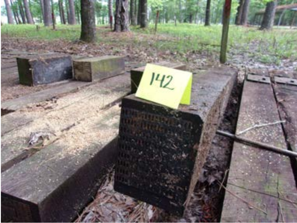
Figure 31 – Tie #142 white oak/DOT/ACZA/oil (Lonza).
