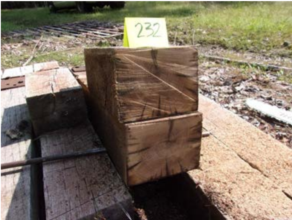
Figure 50 - Tie # 232 white oak/DOT/ACZA/ET (Lonza).
