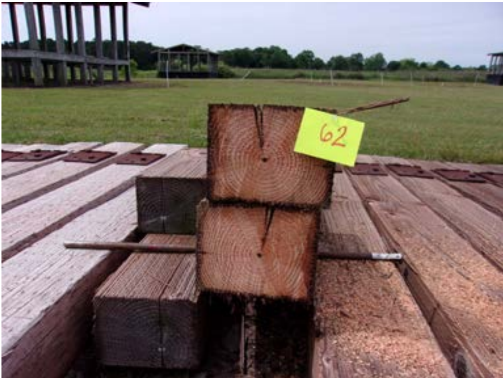
Figure 66 - Tie #62 Douglas fir/DOT/ACZA/ET (Lonza).
