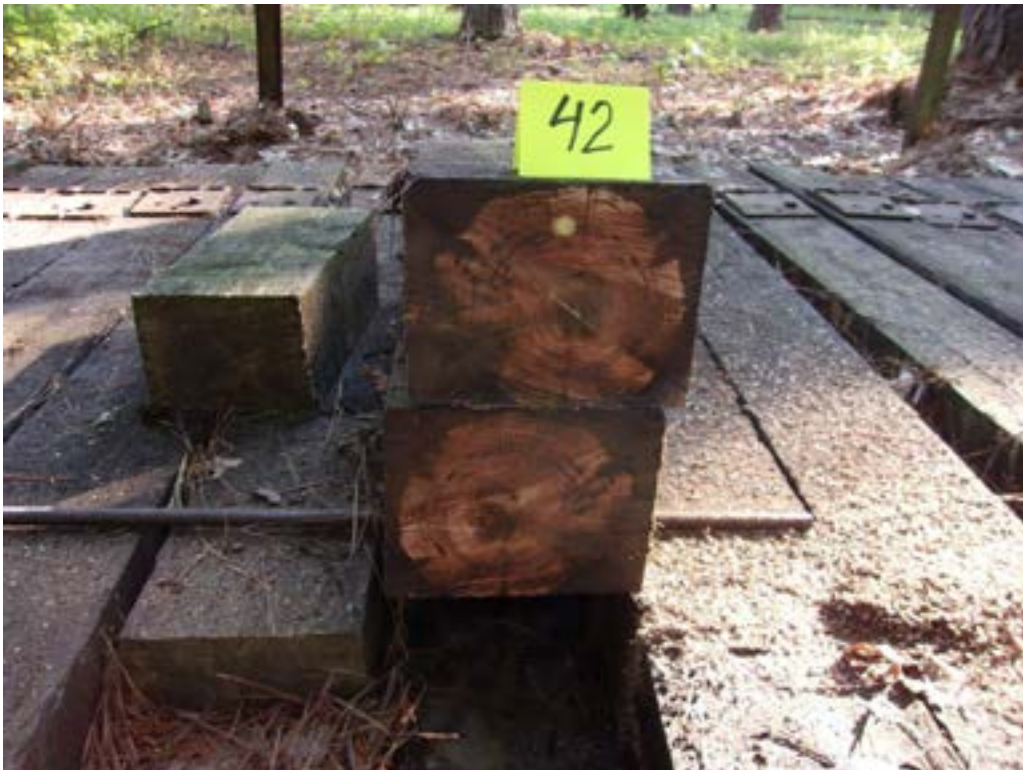
Figure 10 - Tie #42 white oak/borate/creosote 7lbs (Koppers).
