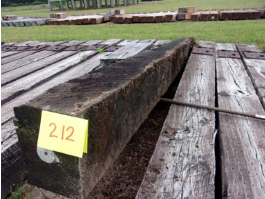
Figure 97 – Tie #212 red oak/borate/creosote 7lbs (Koppers).
