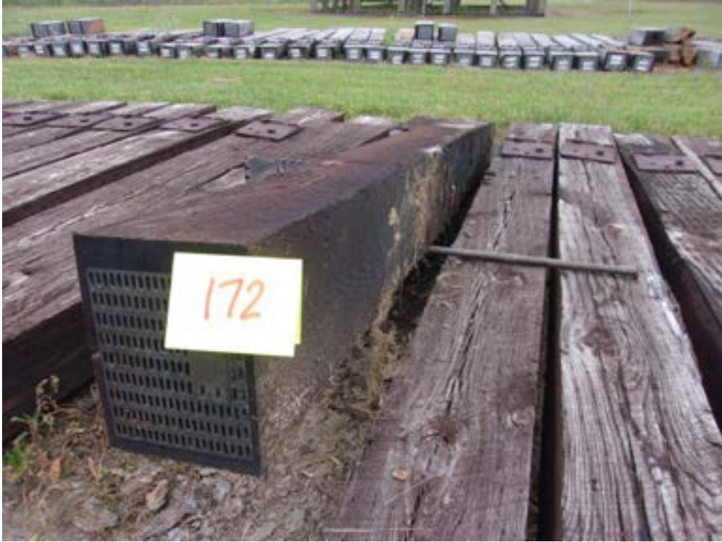
Figure 89 – Tie #172 white oak/DOT/ACZA/oil (Lonza).
