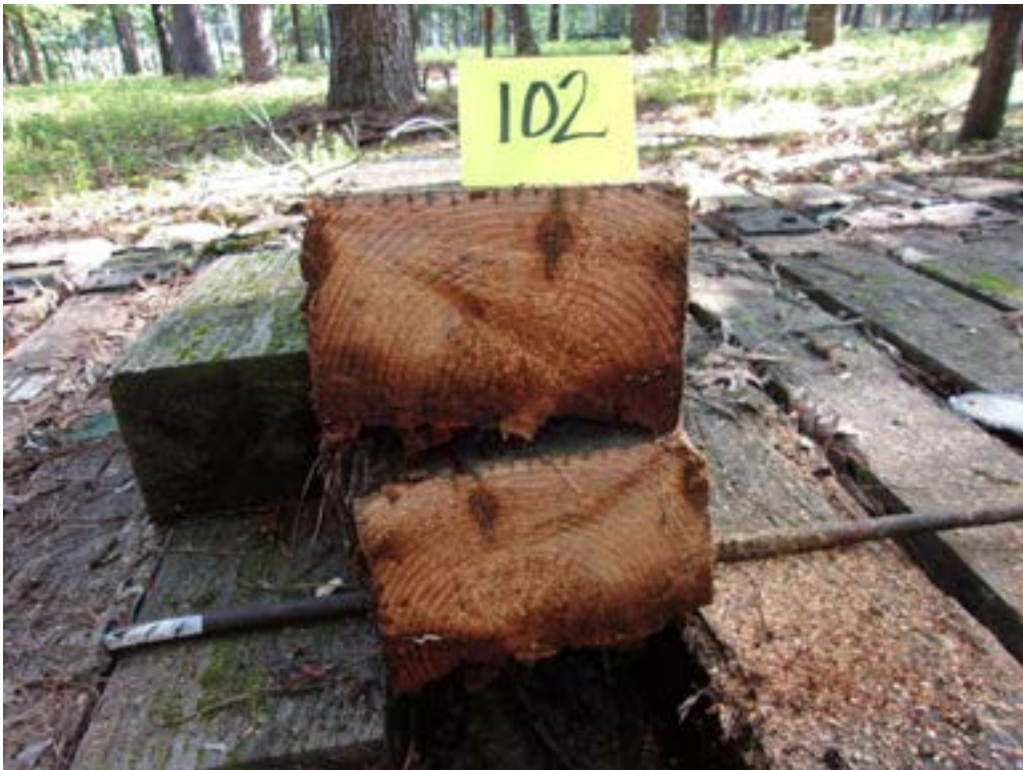
Figure 22 - Tie #102 untreated Douglas fir.
