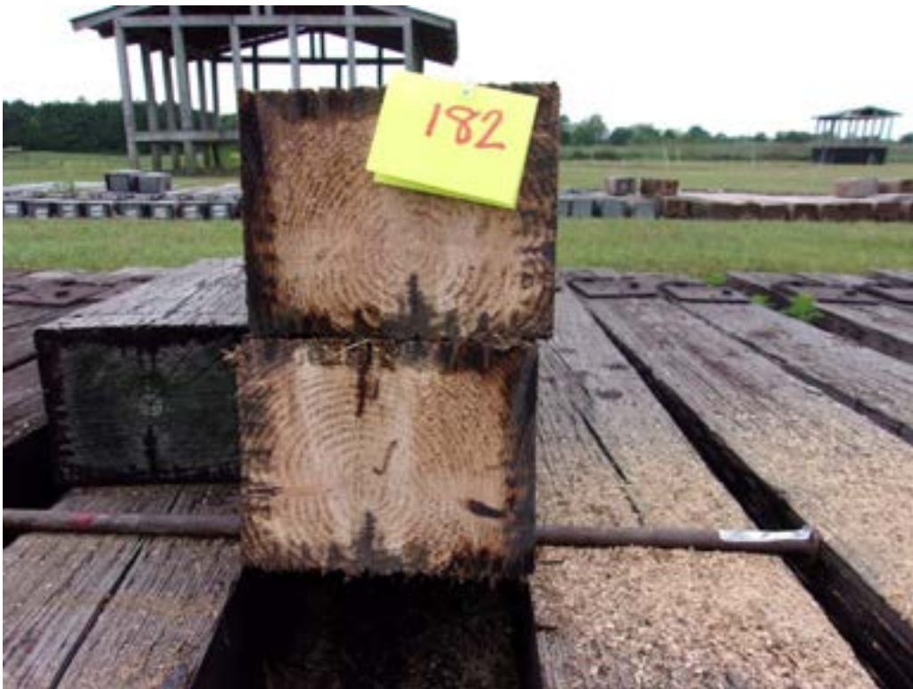
Figure 92 - Tie #182 Douglas fir/P2 (Lonza).
