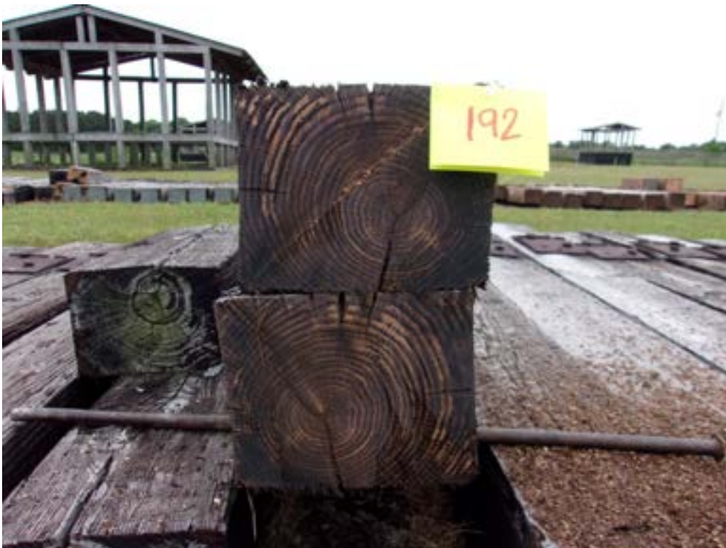
Figure 94 - Tie #192 white oak/borate/creosote 6lbs (Koppers).
