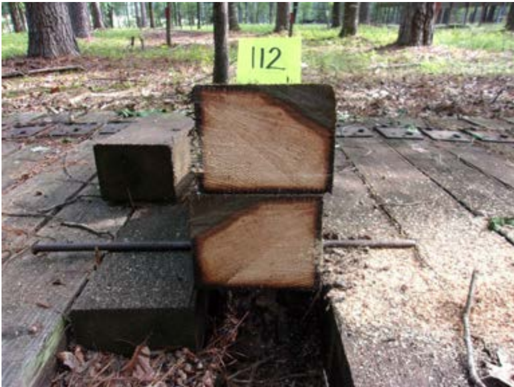
Figure 24 - Tie #112 Douglas fir/DOT/ACZA (Lonza).
