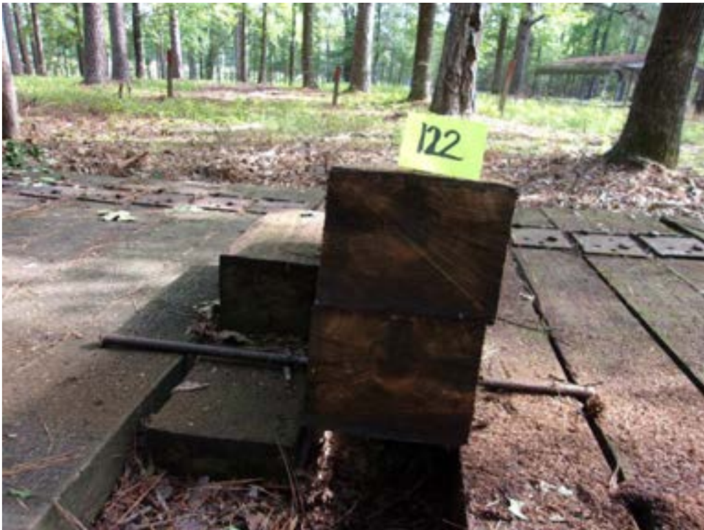
Figure 26 - Tie #122 red oak/DOT/ACZA/oil (Lonza).
