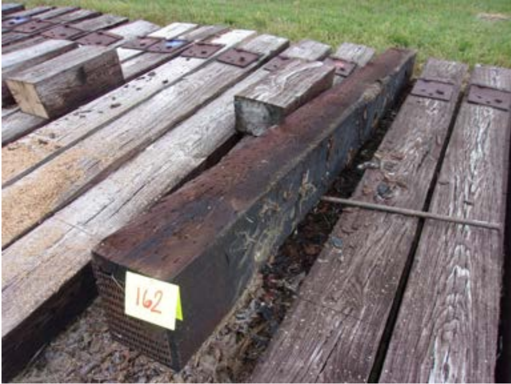
Figure 87 – Tie #162 red oak/DOT/ACZA/oil (Lonza).
