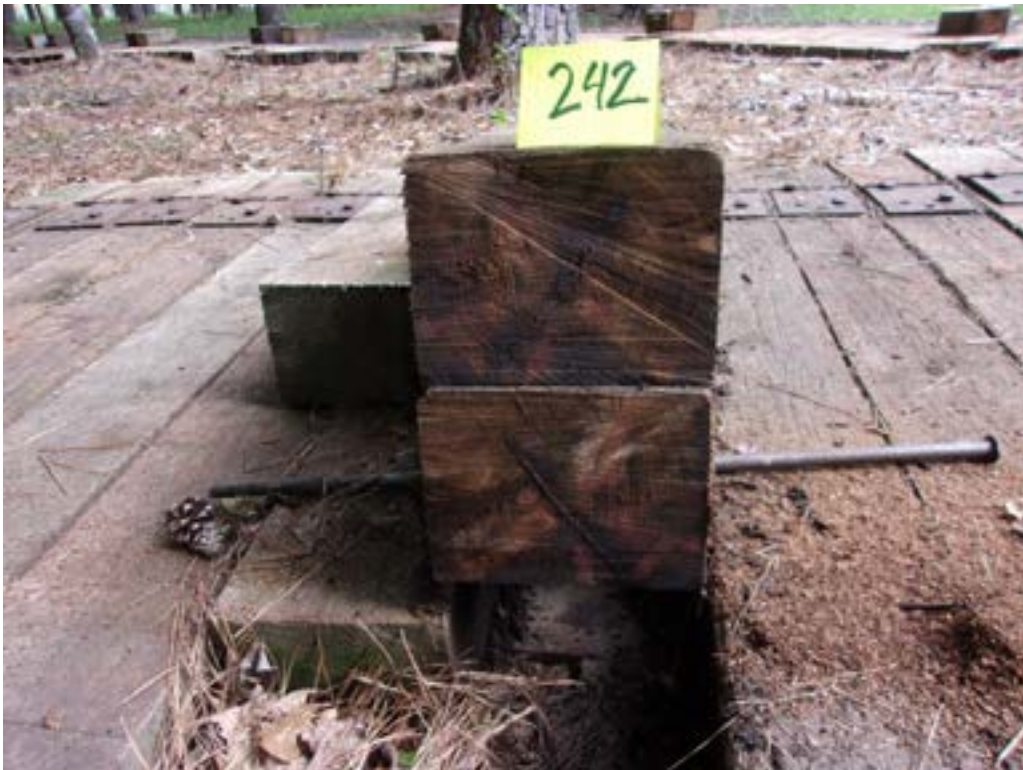
Figure 52 - Tie #242 red oak/ACZA/DOT/ET (Lonza).
