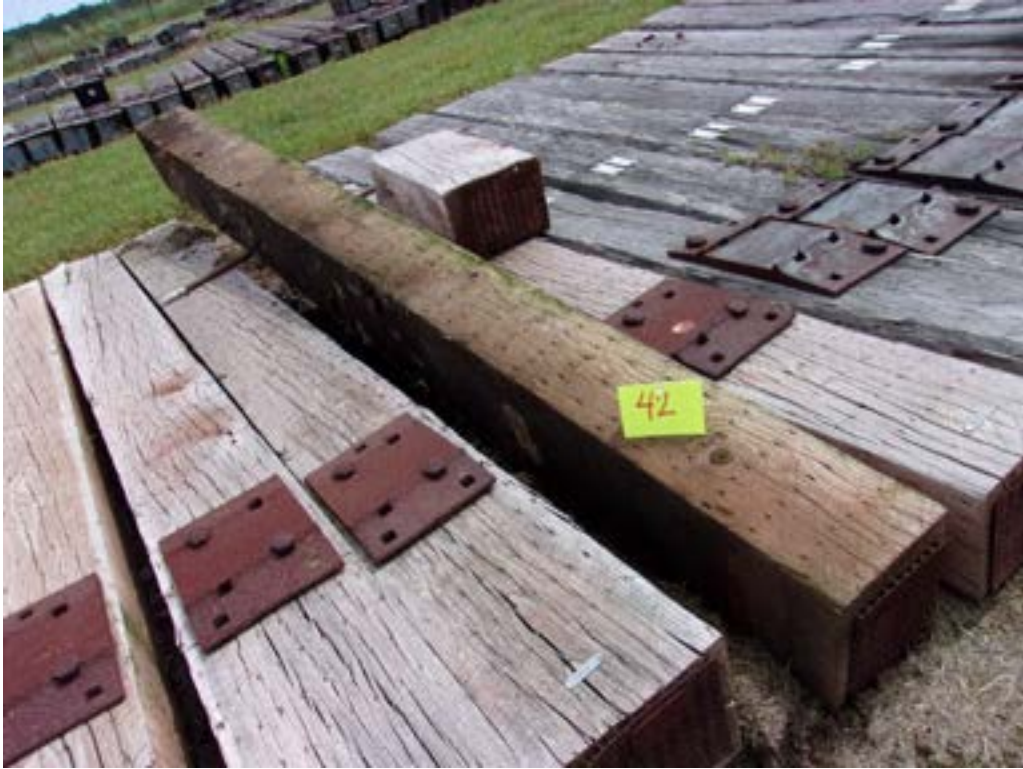
Figure 61 – Tie #42 white oak/DOT/ACZA/ET (Lonza).
