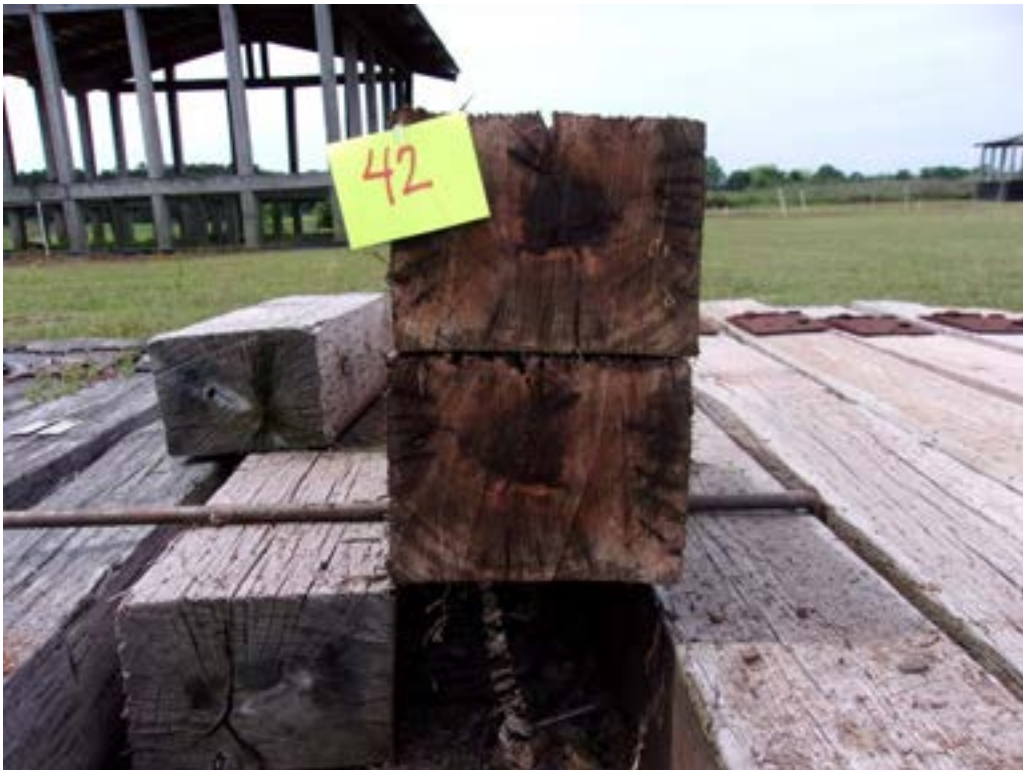
Figure 62 - Tie #42 white oak/DOT/ACZA/ET (Lonza).
