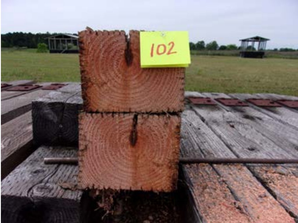
Figure 74 - Tie #102 untreated Douglas fir.
