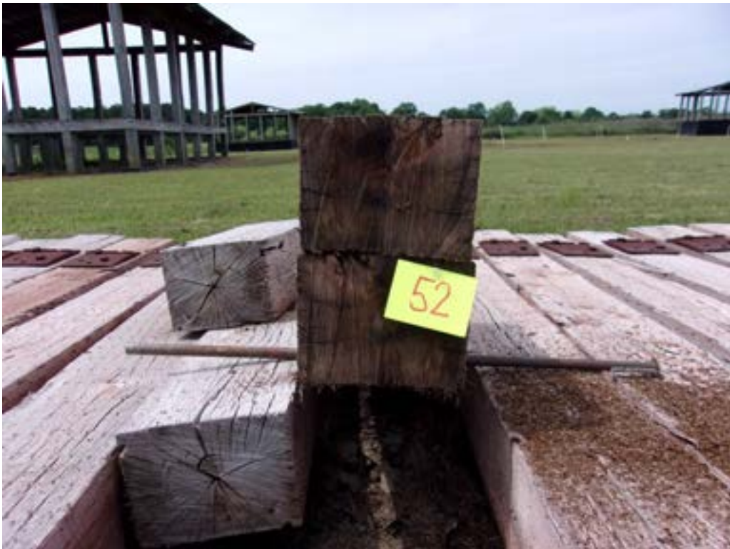
Figure 64 - Tie #52 red oak/DOT/ACZA/ET (Lonza).
