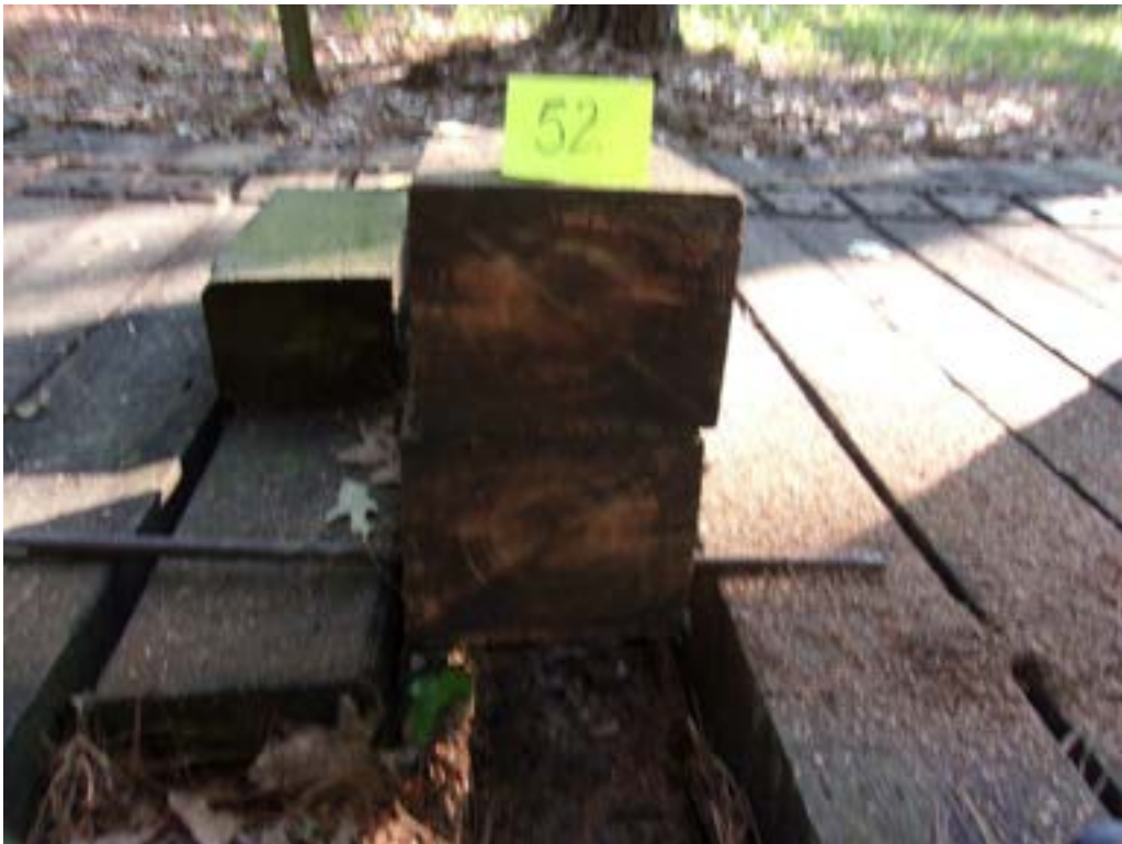
Figure 12 - Tie #52 red oak/borate/creosote 6lbs (Koppers).
