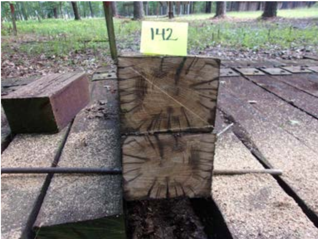
Figure 32 - Tie #142 white oak/DOT/ACZA/oil (Lonza).
