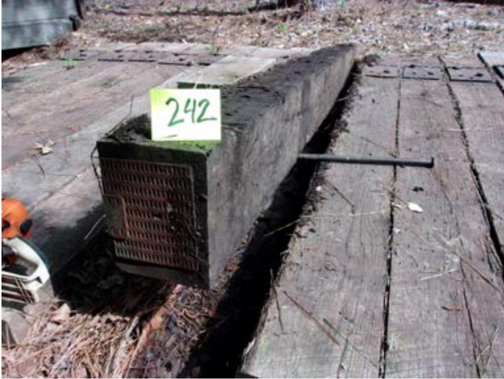
Figure 51 – Tie #242 red oak/ACZA/DOT/ET (Lonza).
