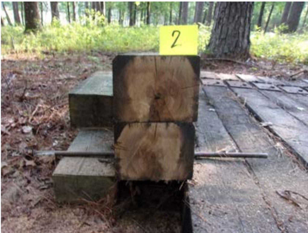
Figure 2 - Tie #2 white oak/borate/creosote 6# (Koppers).
