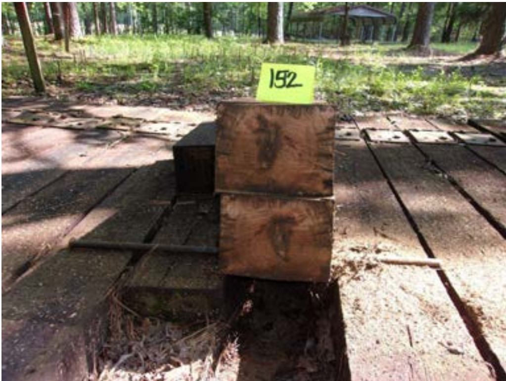
Figure 34 - Tie # 152 red oak/DOT/ACZA/oil (Lonza).
