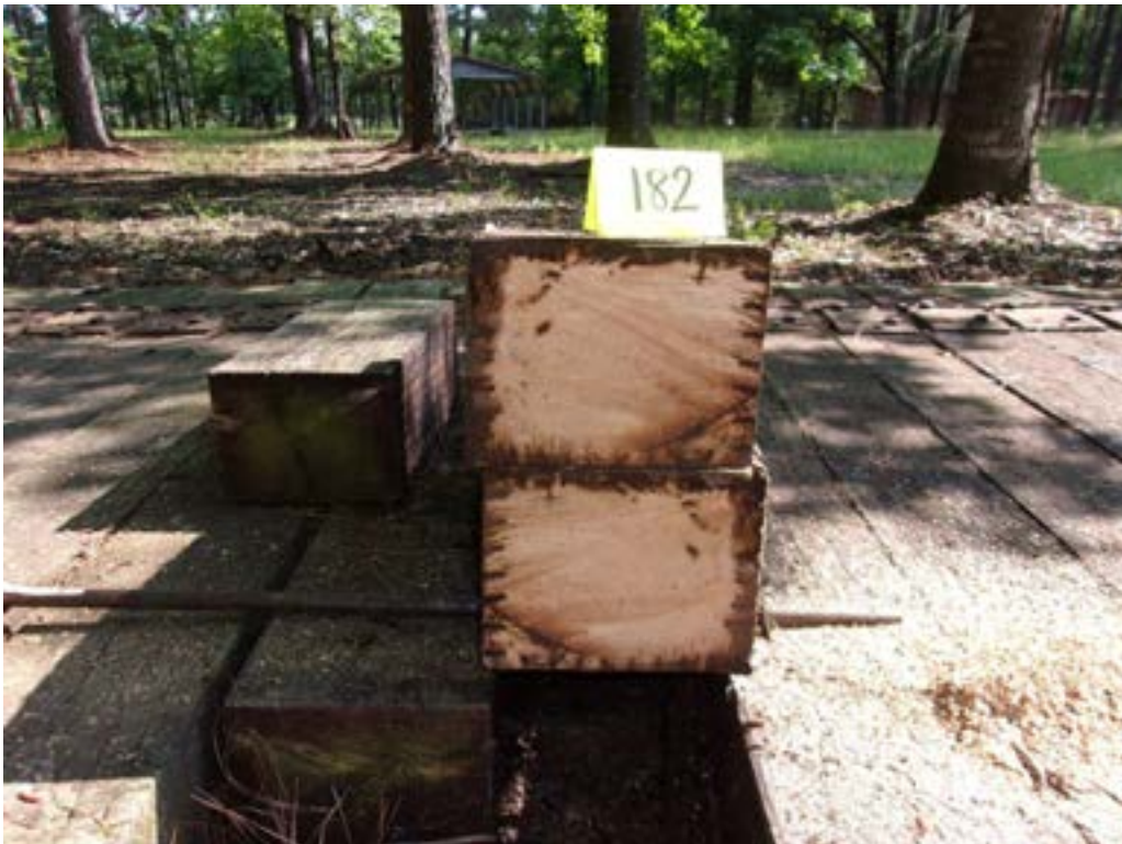
Figure 40 - Tie #182 Douglas fir/P2 creosote (Lonza).
