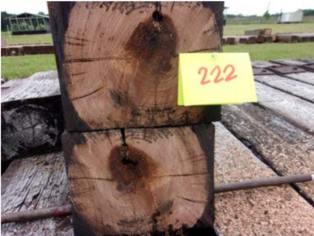
Figure 100 - Tie #222 red oak/borate/creosote 6lbs (Koppers).
