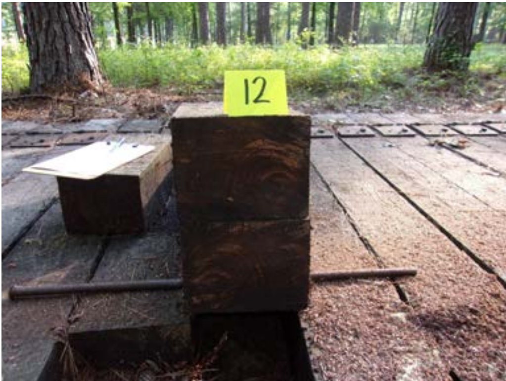
Figure 4 - Tie #12 red oak/borate/creosote 7lbs (Koppers).
