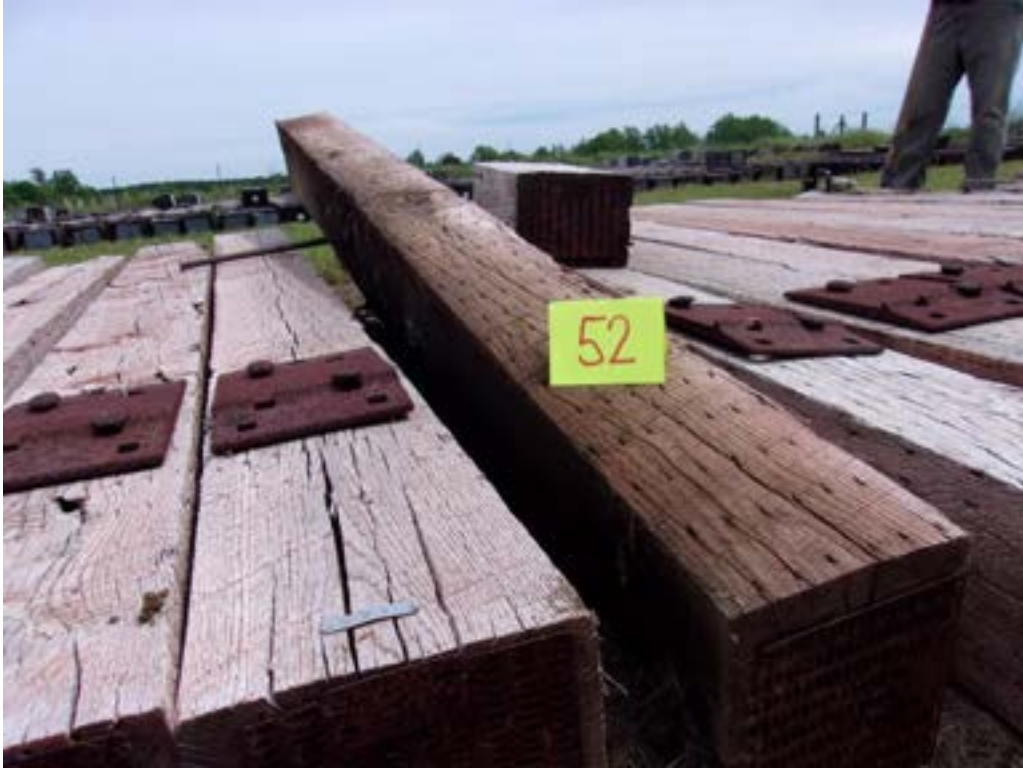
Figure 63 – Tie #52 red oak/DOT/ACZA/ET (Lonza).
