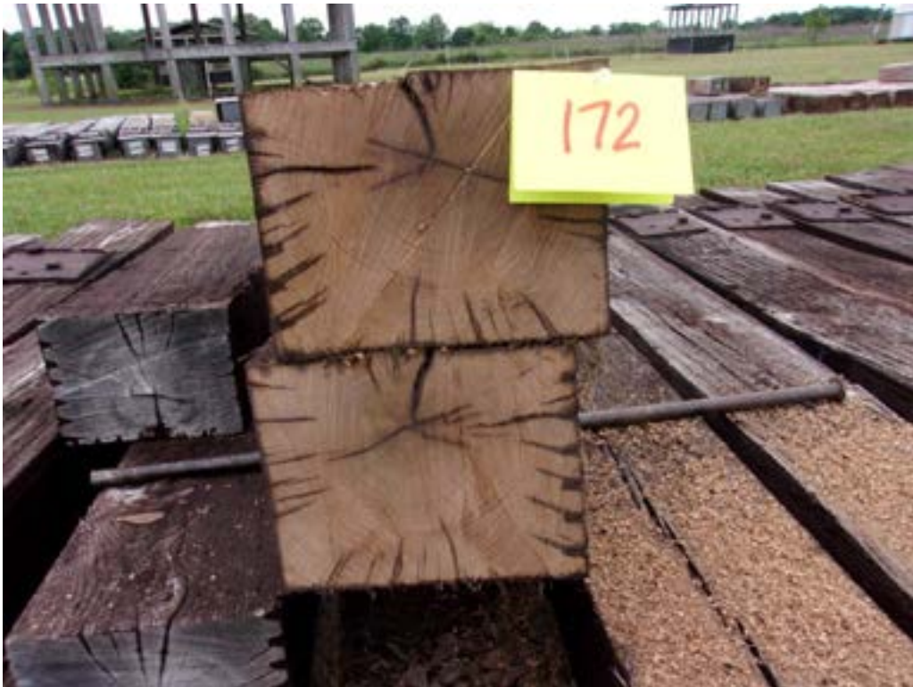
Figure 90 – Tie #172 white oak/DOT/ACZA/oil (Lonza).
