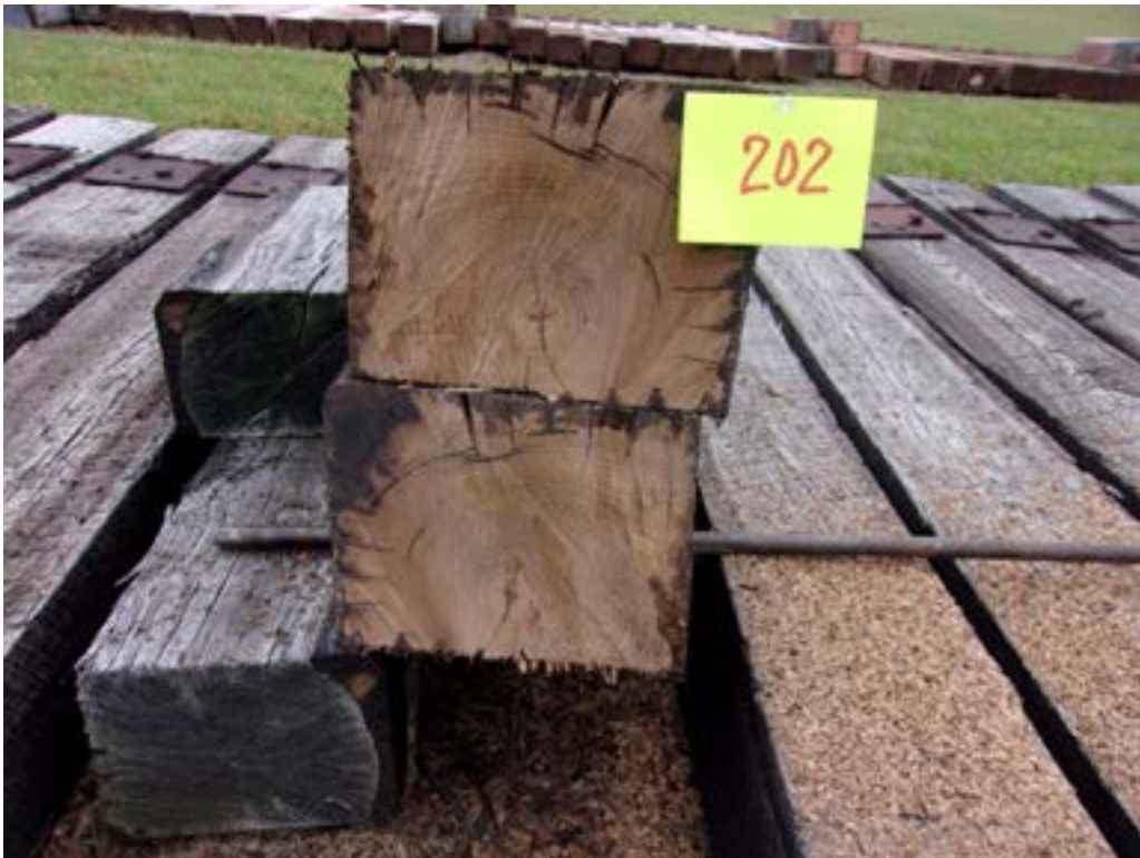
Figure 96 - Tie #202 white oak/borate/creosote 7lbs (Koppers).
