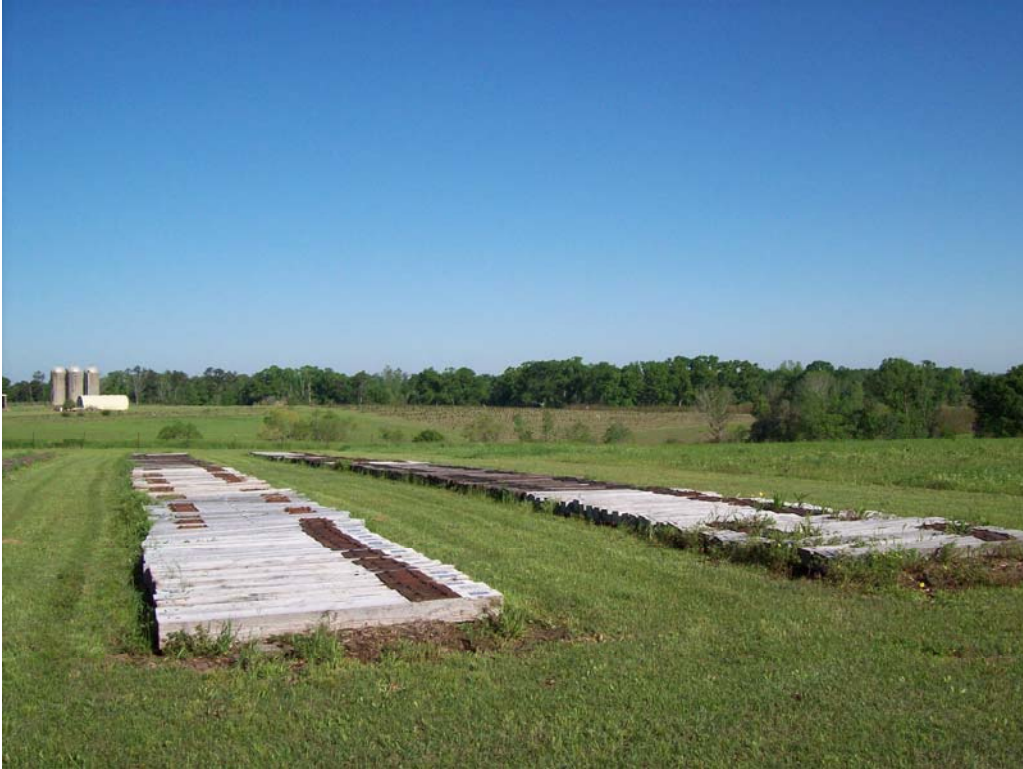
Figure 5 – An overall view of the ties exposed at the MSU Formosan Termite Research Facility at the time of the one-year inspection (Site 1).
