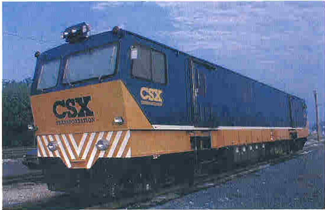
Figure 1A: CSX's GRMS Track Inspection Vehicle.
