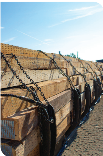
Ties on a tram ready to head into the cylinder for treating.
