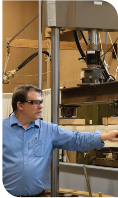
Daniel Hindman, associate professor in wood building design, tests yellow poplar and pine cross laminated timbers for strength.
