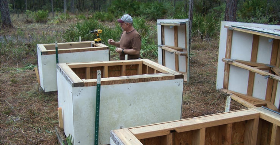
Mike Sanders of Mississippi State University inspects borate-treated structures at the Nisus field test site in Florida. Sanders also oversees the RTA tie field tests in which Nisus uses both Cellutreat and QNAP copper naphthenate treatments.
