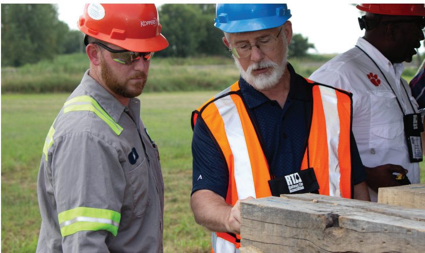
Students concentrate on species and defects as they consider the ties at the plant. Terry Conners discusses a split tie with Koppers' Neal Galford.
