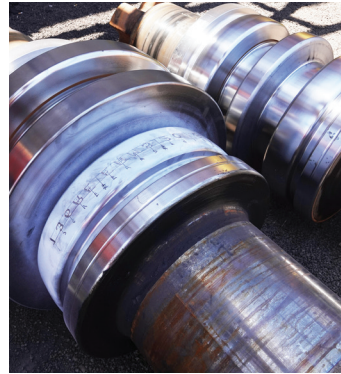
Set of rolling mill finisher rolls, displaying the engraving used to create the rail brand.
