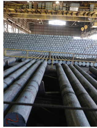
Blooms are loaded on the re-heat furnace charge bed.
