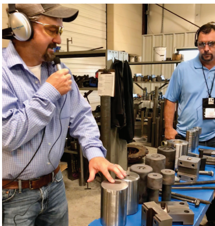
Plant Manager Brett McIntosh shows how Lewis Bolt tooling is made completely in house for various upsetting machines.
