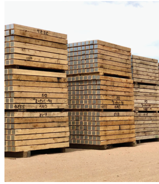
This facility uses stickering rather than German stacking to control air-drying speed in the drier Denver climate.
