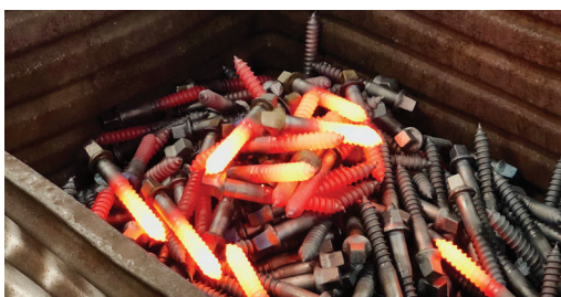
Screw spikes after final step of roll threading.
