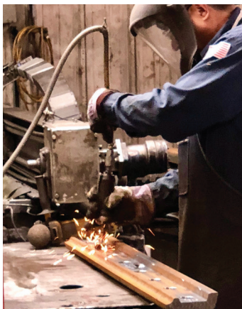
Deburring joint bar after being cut and drilled.
