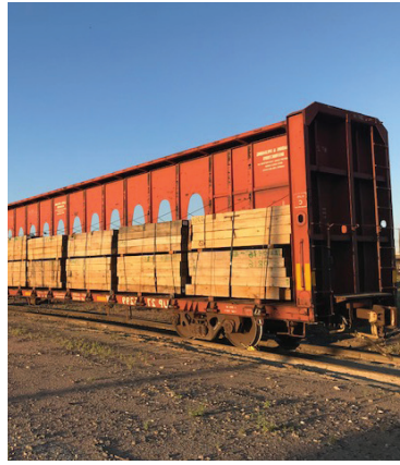
Procured inbound ties on centerbeams heading to the tie unloader.
