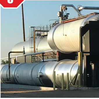
A 165-foot by 8-foot treating cylinder on site at facility.
