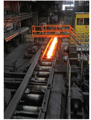
A bloom exiting the re-heat furnace.
