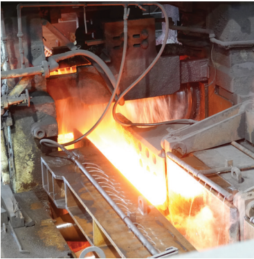
Blooms are being processed at the first breakdown mill stand.
