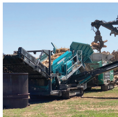
Biomass feedstock (which could include end-of-life ties) is chipped for collection for reactors which produce the biochars.
