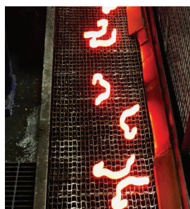
Rail anchors after forming.
