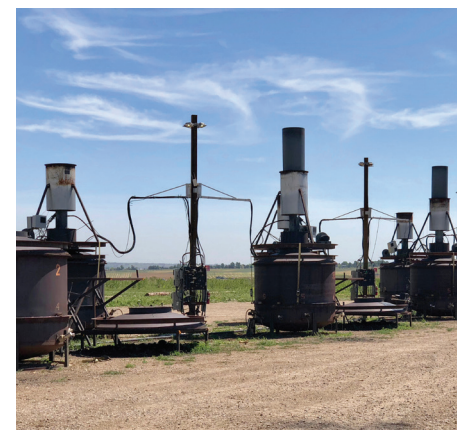
Some of the onsite BioChar NOW! reactors in action.
