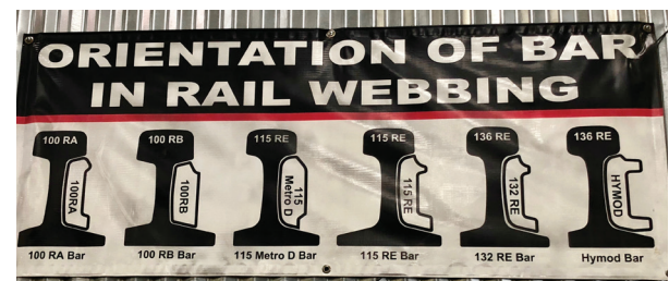
Multiple rail weights and profiles require just as many joint bars.
