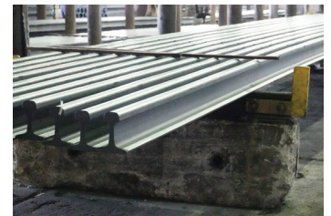
Lift of rails ready to be placed in storage racks for cooling.
