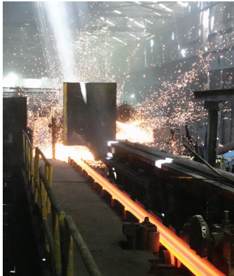
A hot saw is used to cut rails to length.
